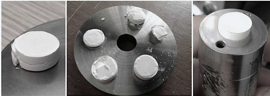
Figure D.4 – Examples of solid samples obtained with the cylindrical mold.
