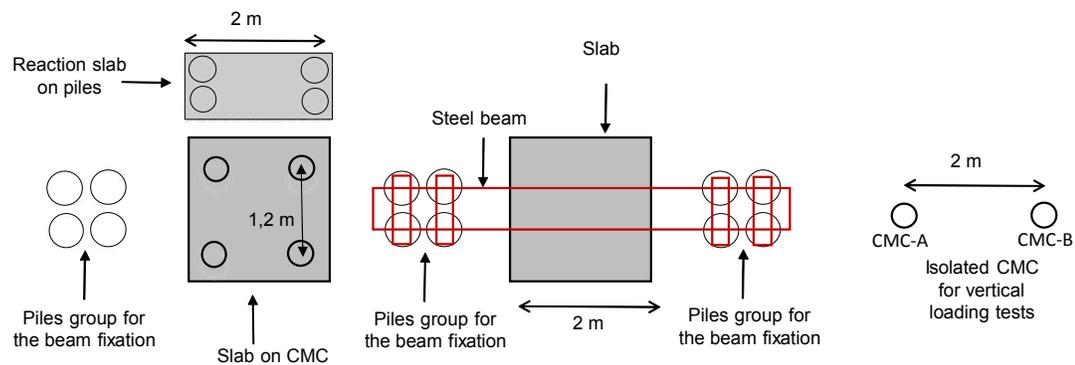
Fig. 3.2. The detail arrangement of the testing site
