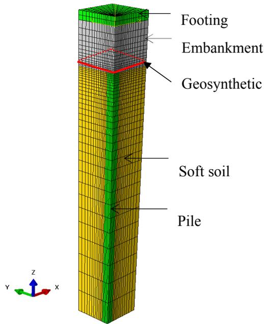
Fig. 5.37. Finite element mesh of the GRPS embankment
