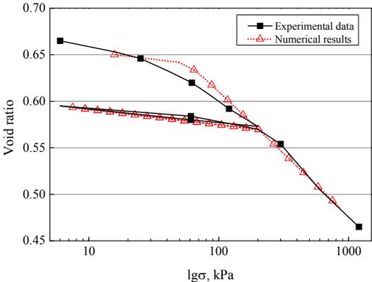
Fig. 3.7. Oedometric tests on the silty clay sample
