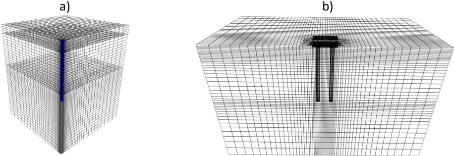
Fig. 3.6. 3D meshes for the numerical analyses: a) single pile; b) unreinforced and reinforced footings
