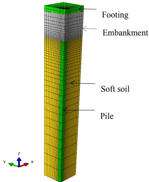
Fig.5.19. Finite element mesh of the piled embankment
