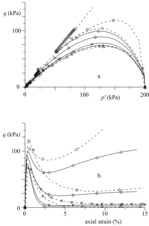
Fig. 4.20. Comparison of simulations and experiments: effect of initial density on triaxial undrained compression tests on Hostun sand with an initial mean effective stress  $p' = 200$  kPa (Gajo and Muir Wood, 1999)
