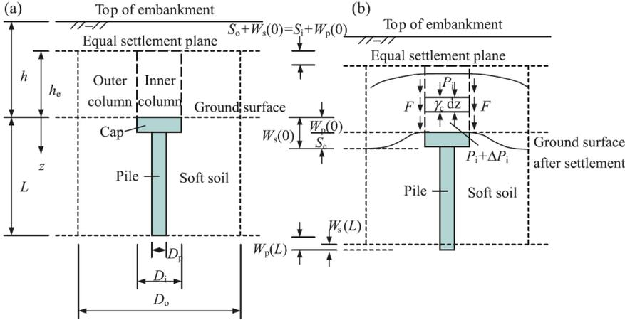
Fig. 1.8. Analytical model for the pile-supported embankment. a) Embankment before settlement; b) Embankment after settlement (Chen et al., 2008)
