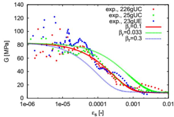
Fig. 4.24. The degradation curve of stiffness versus strain
