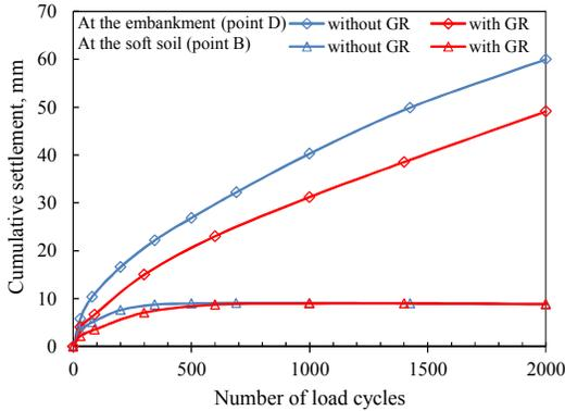
Fig. 5.46. Cumulative settlements under cyclic loading (V = 100 km/h)
