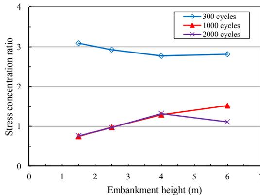
Fig. 5.34. Stress concentration ratio for different embankment heights
