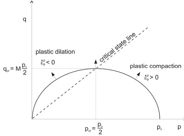
Fig. 2.8. Failure criterion of Cam-clay model (Itasca, 2009)
