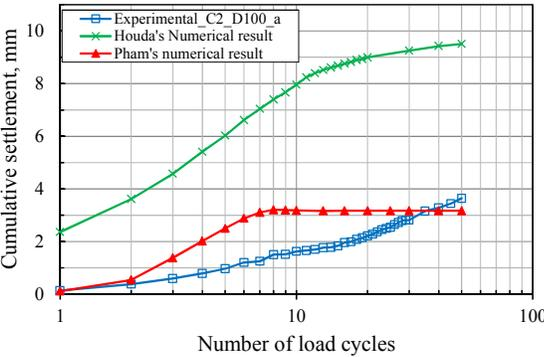
Fig. 5.14. Measured and numerical cumulative settlements for the cyclic test C2\_D100
