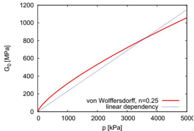
Fig.4.23. The generation of the  $G_0$ - $p$  curve
