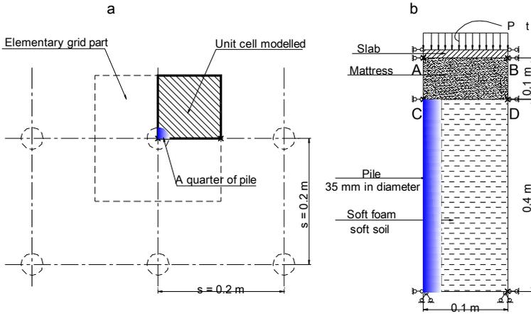
Fig. 5.5. Unit model used for the 3D numerical analyses
