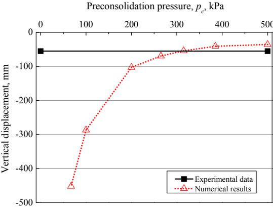
Fig. 3.8. Influence of  $p_c$  on the vertical footing displacement for the unreinforced footing
