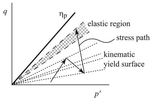
Fig. 4.19. Kinematic hardening Mohr-Coulomb model
