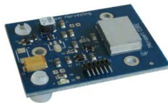
**Fig. 21.** Image of the thermoelectric generator studied (mounted on the board and without the heat sink).
