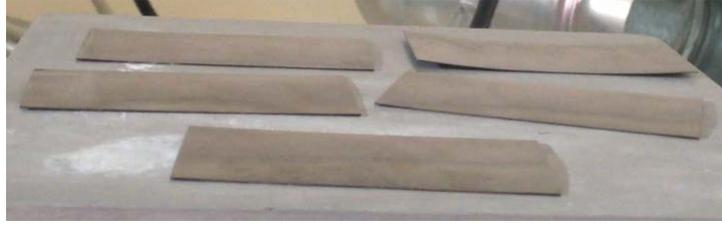
**Fig. 24.** (a) 4K hysteresis bimetals deposited on hot plate to check their bistability, (b) bimetals curvature at ambient temperature 25°C, (c) Bimetals curvature at their snapping temperature (87°C).
