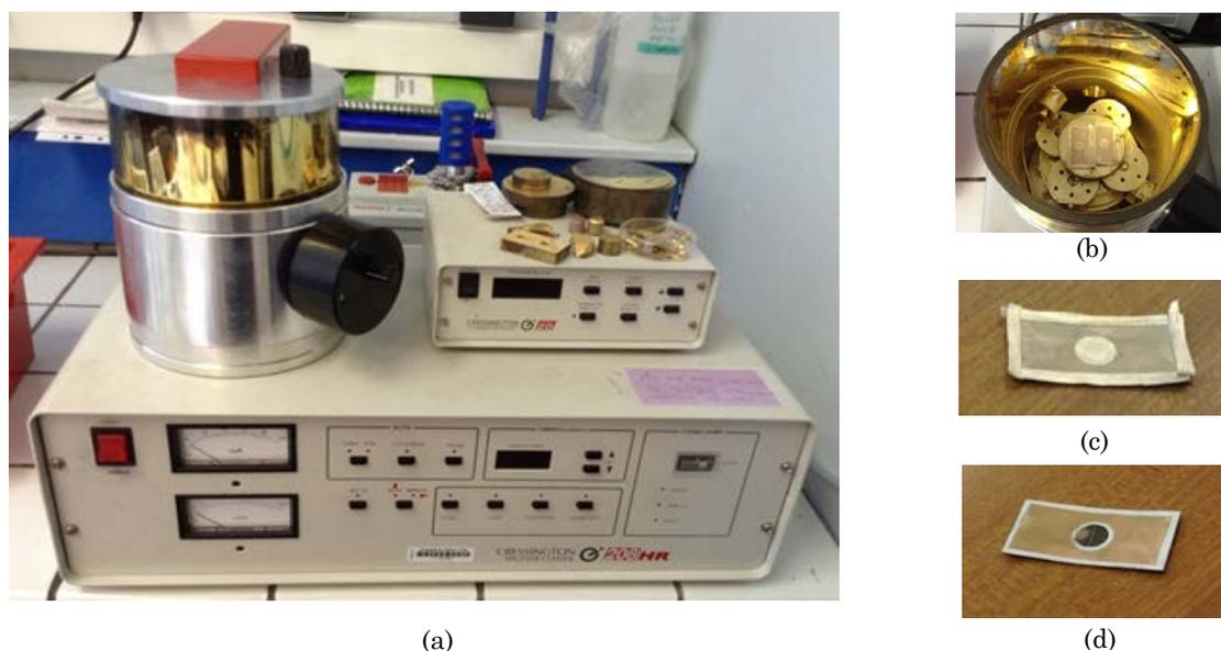
**Fig. 4.** (a). Cressington Sputter coater 208HR used for the PVD gold electrode deposition, (b,c). bimetals after the electroding step, (d) bimetal after the mask removal.
