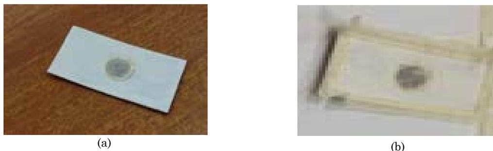
**Fig. 3.** (a). mask on the hallmark of the bimetal, (b). Mask on the bimetal's hallmark and sides.
