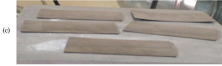
Fig. 24. (a) 4K hysteresis bimetals deposited on hot plate to check their bistability, (b) bimetals curvature at ambient temperature 25°C, (c) Bimetals curvature at their snapping temperature (87°C).
