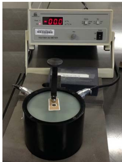
Fig. 6. Experimental setup used to measure d_{33} coefficient of each sample (in this picture the sample has not been poled yet).
