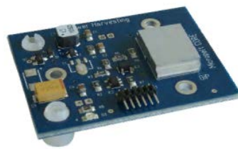
Fig. 21. Image of the thermoelectric generator studied (mounted on the board and without the heat sink).
