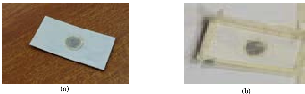
Fig. 3. (a). mask on the hallmark of the bimetal, (b). Mask on the bimetal's hallmark and sides.
