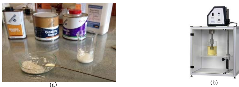
Fig. 1. (a). Different constituents needed for the preparation of the piezoelectric paint, (b). Ultrasonic processor Hielscher UP400S used for the paint homogenization.
