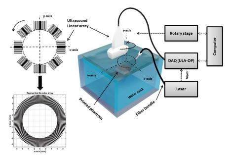
FIGURE 6.1: Annotated schematic of optoacoustic experimental setup. The ultrasonic probe is mounted on the rotary stage (not depicted). The scanning is taking place over the sample (printed phantom) located parallel to the plane of imaging under the array of sensors within the water tank. The water tank is aligned with the x-y axes of Cartesian coordinate system. The z-axis is corresponding to the axis of rotation.
