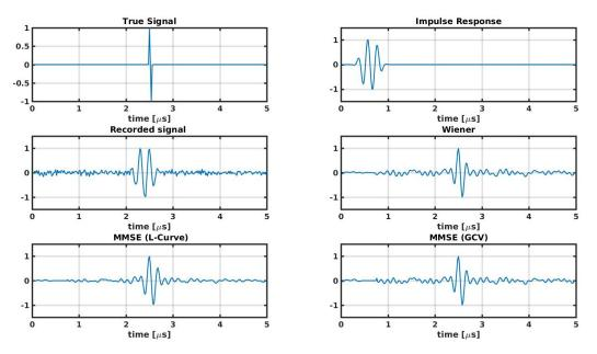
FIGURE 5.1: The effect of acousto-electric impulse response (AIR) on the recorded signal and three method of deconvolution to retrieve the original signal in the presence of -10 dB noise.
