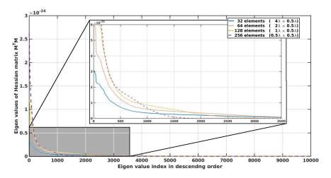
FIGURE 4.5: Eigenspectra of the hessian matrices for the transfer matrix of four virtual arrays. The highlighted region has been magnified for better visualization.
