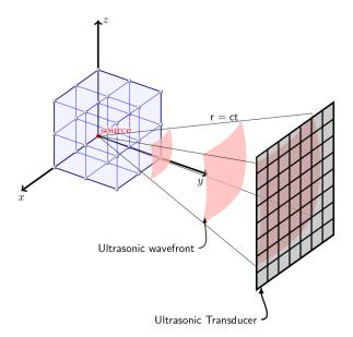
FIGURE 3.3: Depiction of the emanating wave from a source (shown by red) in the discretized FOV (blue lattice) and it's intersection with the surface of ultrasonic transducer. Only the portion of spherical wave that is intersecting with the active area of transducer is presented. The rest of spherical wave is not being sensed by the transducer and that, the finite size of the aperture introduces a low pass filter with cutoff in the angular frequencies to the source wave.
