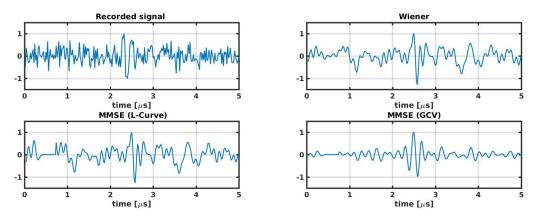
FIGURE 5.2: The comparison between the performance of deconvolution approaches for retrieving the original signal in the presence of -10 dB noise.
