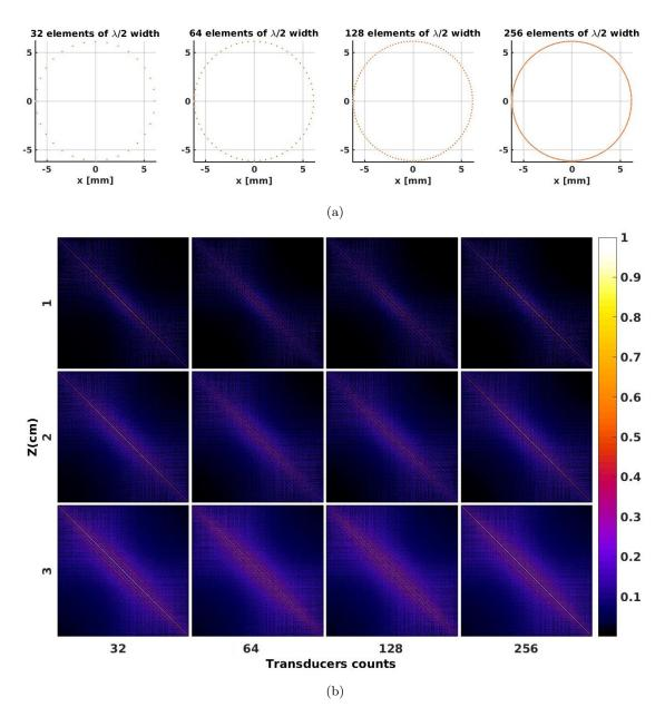
FIGURE 4.3: (a) Schematic of four annular arrays differ in number of elements and inter-element spacing and (b) their crosstalk talk matrices for three xy-planes parallel to the aperture situated at the axial distances (depths) respectively at 1, 2 and 3 cm away from the aperture. The crosstalk matrices are normalized w.r.t the maximum element in each matrix.
