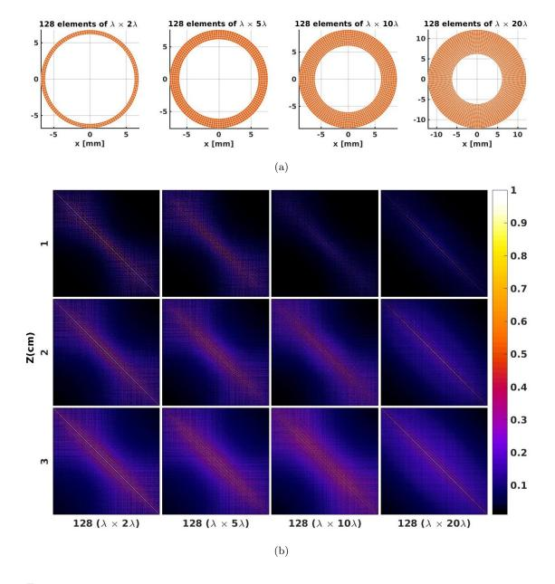
FIGURE 4.7: (a) Schematic of four segmented annular arrays of 128 elements varying in element height. (b) The corresponding crosstalk matrix for three axial plane away from the aperture. It is clear that for the aperture with larger elements, the diagonal elements are stronger and off-diagonal elements are much weaker.
