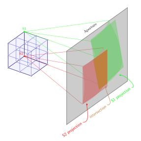
FIGURE 4.1: The projection of emanated waves from two source located in voxels apart over the surface of detecting aperture. The brown region represents the intersection area between the projection of two sources.
