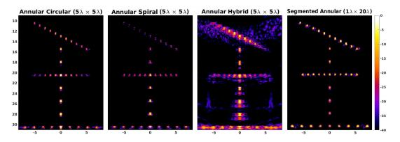
FIGURE 5.12: The VE-WDSBP reconstructed B-mode images of the point reflectors.
