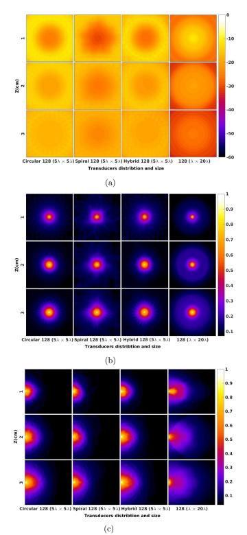
FIGURE 4.12: Qualitative comparison on the effect of the geometrical distribution based on (a) 60 dB sensitivity map, (b) spatial aliasing for the central pixel and (c) spatial aliasing for the marginal pixel. The sparser aperture is, the lesser aliasing but lesser overlapping energy as well.
