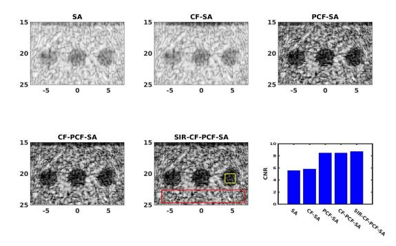
FIGURE 5.7: The effect of weighting factors in ameliorating the contrast of anechoic cyst of 3 mm  $\oslash$  and plot of their CNR values. The B-mode images are simulated with FMC approach and reconstructed with SAFT technique. The yellow and red frames are indicating the areas have been used for calculation of the CNR.
