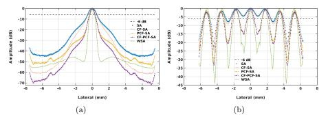
FIGURE 5.6: Logarithmic profile of the scatterers (a) at the depth of 27 mm and (b) at the depth 32 mm away from the transducer, weighted with different weighting factors.
