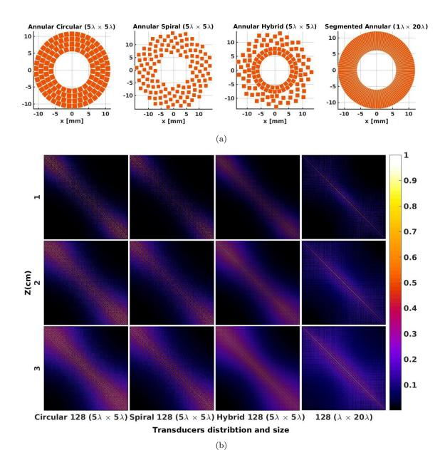
FIGURE 4.11: (a) Schematic of virtual annular arrays of 128 elements varying in geometrical distribution. (b) The corresponding crosstalk matrix for three axial planes away from the aperture.
