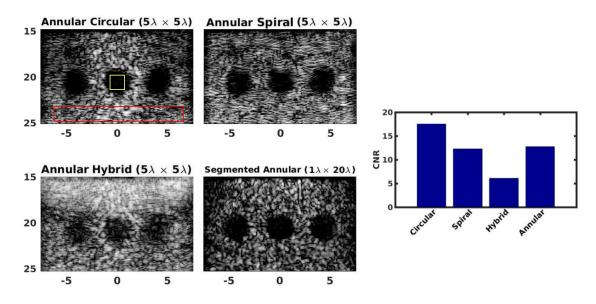
FIGURE 5.14: Evaluating the PE performance of the four virtual arrays based on the contrast and energy distribution. The yellow and red frames are indicating the lesion and background area used for calculating the CNR.
