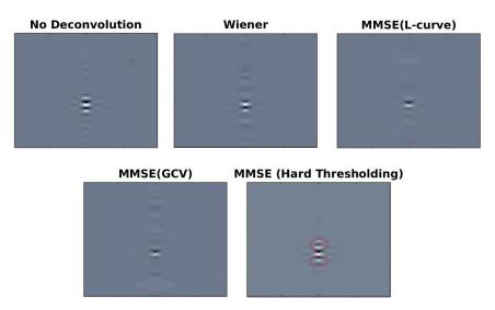
FIGURE 5.4: The comparison between four deconvolution approaches in the reconstructed image. The hard thresholding has lesser value for the lumpy background due to suppression of the noise yet with artifacts indicated by the red circle.
