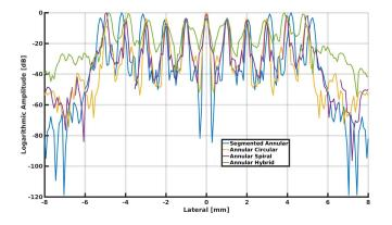
FIGURE 5.13: The lateral profile of the reconstructed images for each of the arrays at the range of 20mm.
