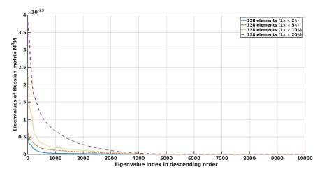
FIGURE 4.9: Eigenspectra of the hessian matrices for the transfer matrix of four virtual arrays, varying in the height of element.
