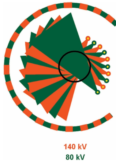
Figure 2.3: Principle of fast kV switching systems to acquire dual-energy CT data. Figure from [Heismann et al., 2012]. Low (green) and high (orange) voltage projections are acquired at consecutive projection angles.
