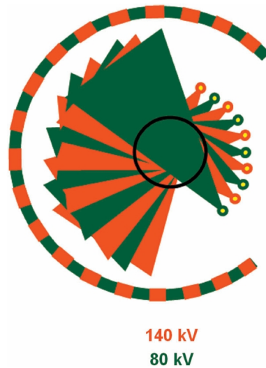
Figure 2.3: Principle of fast kV switching systems to acquire dual-energy CT data. Figure from [Heismann et al., 2012]. Low (green) and high (orange) voltage projections are acquired at consecutive projection angles.
