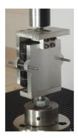
Figure 2. 14: Transverse shearing test device for interlock reinforcement [CHA 12]
