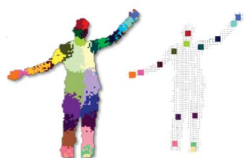
(c) A depth image based pose estimation (frame extracted from [259])
