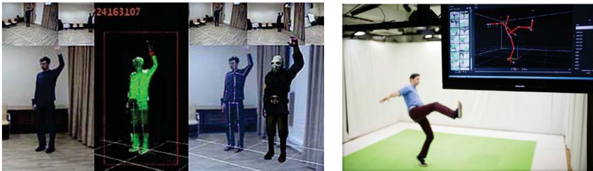
Fig. 1.2 Examples of commercial markerless motion capture systems from MetaMotion 2 ( left ) and OrganicMotion 3 ( right ).
