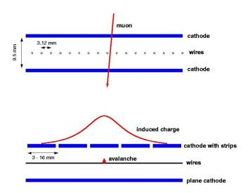
Figure 2.31: Orthogonal section of a cathode strip chamber.
