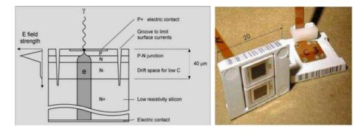
Figure 2.19: Left: APD layout. Right: Photo of APDs.
