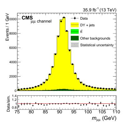
Figure 4.15:  $Z \to \mu^+\mu^- Z \to \mu\mu$  events in the low- $m_{\ell\ell}$  CR after application of trigger, ID, isolation, and DY normalization SFs and momentum corrections. The uncertainty bands on the simulated background histograms only include statistical uncertainties. The uncertainty bars in the ratio plots represent the combined statistical uncertainties of data and simulation.
