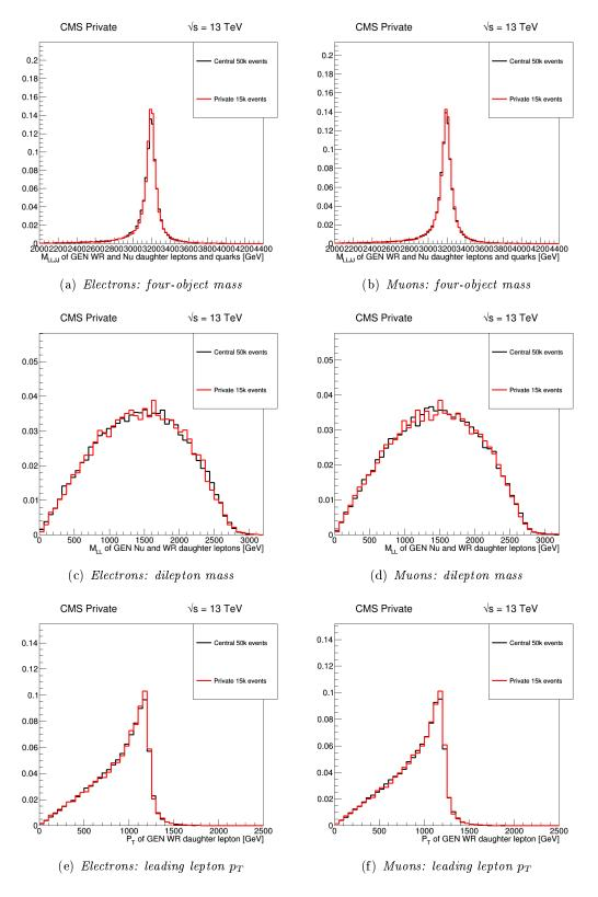
Figure 4.4: Comparison of produced signal samples with the official 2015 ones for  $m_{W_R} = 3200 \text{ GeV}$  for different kinematic variables in both electron (on the left) and muon (on the right) channels.
