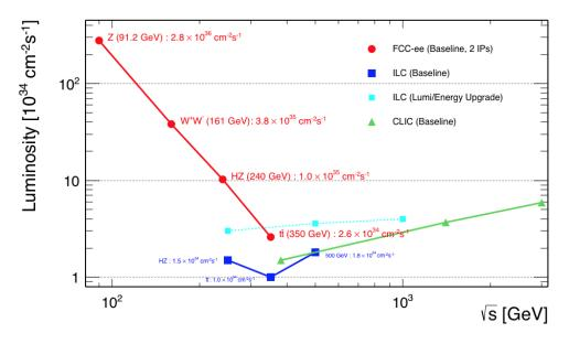
Figure 5.19: Luminosity as a function of mass for different experiments.
