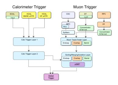
Figure 2.33: Scheme of the L1 trigger system.
