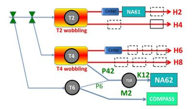
Figure 3.9: Layout of the SPS secondary beam line: the 400 GeV primary proton beam is split into three beams directed towards the T2, T4, and T6 targets. Thanks to the T2 "Wobbling station", the two H2 and H4 secondary beams are derived.
