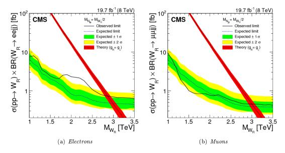
Figure 1.4: The 95% CL exclusion limit for  $W_R$  boson production cross section times branching fraction, computed as a function of  $m_{W_R}$  assuming the right-handed neutrino has half the mass of the  $W_R$  boson, for the 8 TeV analysis. The signal cross section PDF uncertainties (red band surrounding the theoretical  $W_R$  boson production cross section curve) are included for illustration purposes only.
