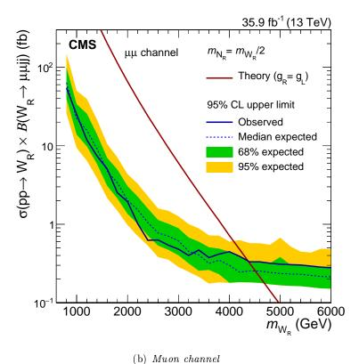
Figure 4.41: Expected and observed 95% CL upper limits on the product of  $\sigma(pp \to W_R)$  and branching fraction  $B(W_R \to \ell \ell jj)$ . The inner (green) band and the outer (yellow) band indicate, respectively, the expected 68% and 95% CL exclusion regions.
