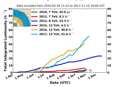
Figure 2.7: Cumulative integrated luminosity delivered by LHC to CMS during stable beams for proton-proton collisions in different years of data taking.
