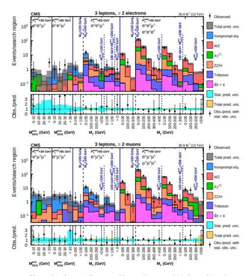
Figure 5.1: Observed and expected event yields as a function of  $M_{2\ell OS}^{min}$  and  $M_T$  for events with at least two electrons (top), and with at least two muons (bottom) in the trilepton channel. The contribution of each background source is shown. The first 8 bins of each figure correspond to the low-mass region, while the rest displays the high-mass region. [170]
