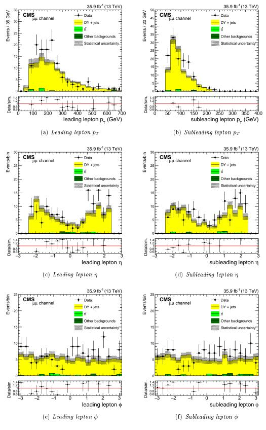
Figure 4.35: Comparison between data and simulation of different kinematic variables for muon events with  $m_{\ell\ell jj} > 2.5$  TeV in the low- $m_{\ell\ell}$  CR.
