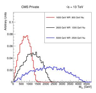
Figure 4.16: Dilepton mass of leptons at generator level from the  $W_R$  decay chain for different  $m_{W_R}$  values. The area under each curve is normalized to 1.
