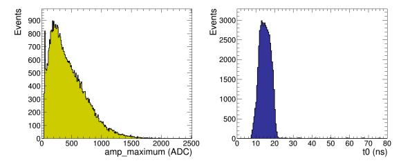
Figure 3.18: Amplitude (on the left) and time (on the right) of the MCP.
