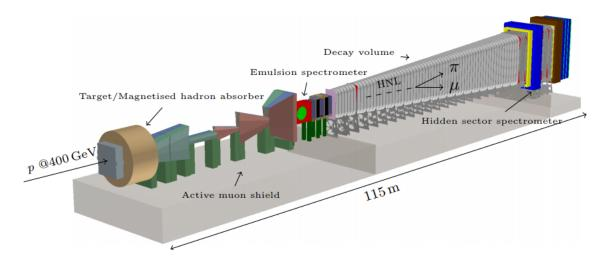
Figure 5.8: Layout of the SHiP detector.
