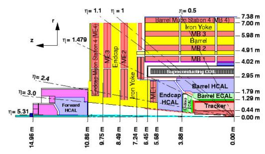
Figure 2.28: Schematic view of the detector showing the different  $\eta$  coverage of the various parts of the HCAL.
