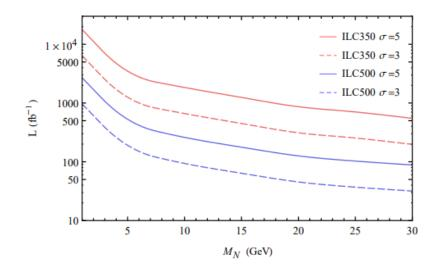
Figure 5.26: Integrated luminosity necessary for observing the Majorana neutrino at the  $3\sigma$  (dashed line) and  $5\sigma$  (solid line) levels at ILC with  $\sqrt{s} = 350$  GeV (red) and  $\sqrt{s} = 500$  GeV (blue) [200].
