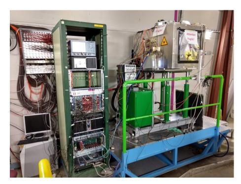
Figure 3.13: Picture of the test beam setup: the digitizer is on the left, while on the right there is the box in which the crystal matrix, the VFE and FE boards are installed.
