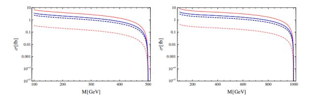
Figure 5.28: Production cross section of the  $e^+e^- \to n\bar{u}_l N_l$  process, followed by the decays  $N \to lW$  ( $l=e,\mu,\tau$ ) and  $W \to q\bar{q}'$ , as a function of the heavy neutrino mass at  $\sqrt{s}=500~{\rm GeV}$  on the left and at 1 TeV on the right [200].
