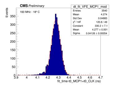
Figure 3.26: Time difference distribution between C3 crystal and MCP1 for a run at 200 GeV. The Gaussian fit is represented by the red line.
