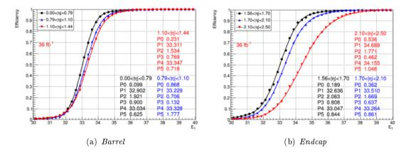
Figure 4.9: Efficiency of electrons passing offline ID requirements to match a L1 candidate with  $E_T > 33 \text{ GeV}$  as a function of  $E_T$  [86].
