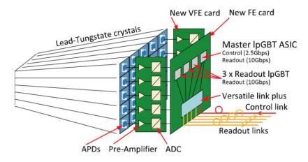
Figure 3.5: Layout of the phase 2 system.
