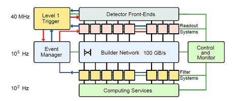
Figure 2.35: Scheme of the DAQ system.
