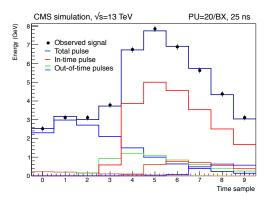
Figure 2.21: Example of fitted pulses for simulated events with 20 average pileup interactions and 25 ns bunch spacing, for a signal in the barrel (left) and in the endcaps (right). Dots represent the 10 digitized samples, the red distributions (other light colors) represent the fitted in-time (out-of time) pulses with positive amplitude. The dark blue histograms represent the sum of all the fitted contributions.
