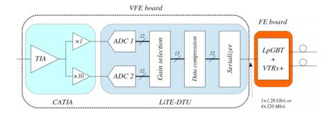
Figure 3.4: Layout of the new electronics for phase 2.
