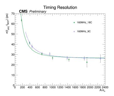
Figure 3.32: Time resolution given by the difference between a crystal and the second MCP as a function of the normalized amplitude for 160MHz and  $18^{\circ}/9^{\circ}$  C.
