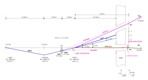
Figure 3.10: Detail of the H4 beam line, produced by the proton beam targeting the T2 target.
