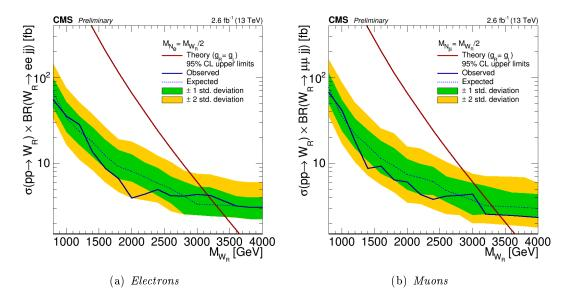
Figure 1.8: The 95% CL exclusion limit for  $W_R$  boson production cross section times branching fraction, computed as a function of  $m_{W_R}$  assuming  $m_{N_R} = \frac{1}{2} m_{W_R}$ , for the 2015 analysis.
