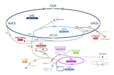
Figure 2.3: CERN accelerator complex.
