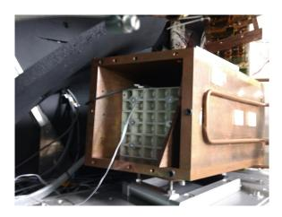
Figure 3.11: Picture of the matrix of  $5 \times 5$  crystals used for the test beam.
