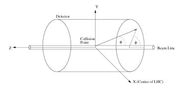
Figure 2.11: Coordinate system of the CMS detector.
