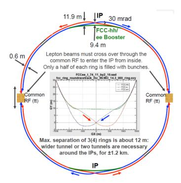
Figure 5.17: Layout of the FCC collider.
