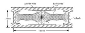
Figure 2.30: Section of a drift tube cell.
