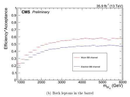
Figure 4.18: Acceptance  $\times$  efficiency for  $W_R \to \ell\ell jj$  events as a function of  $W_R$  mass, in the hypothesis of  $m_{N_R} = \frac{m_{W_R}}{2}$ .
