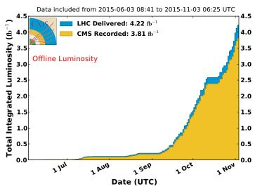
Figure 2.4: Integrated luminosity delivered by the LHC (in blue) and recorded by CMS (in yellow) in 2015 proton-proton collisions.
