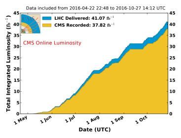
Figure 2.5: Online integrated luminosity (values published by CMS at the time of data taking, not including any later improvements in the calibration) delivered by the LHC (in blue) and recorded by CMS (in yellow) in 2016 proton-proton collisions.
