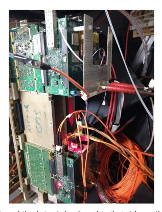
Figure 3.12: Picture of the electronic boards used in the test beam: the VFE board is on the bottom left, next to it there is the VFE adapter to the custom-made FE board, placed transversely. The VFE adapters and the custom-made FE boards will be replaced with the final FE prototype.
