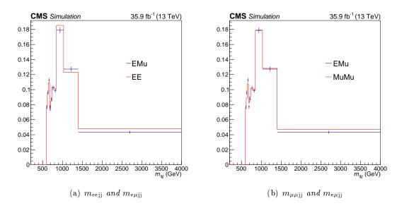
Figure 4.21: The  $m_{\ell\ell jj}$  distribution for simulated e $\mu jj$  events in the flavour-sideband CR and for eejj ( $\mu \mu jj$ ) events in the signal region on the left (right).
