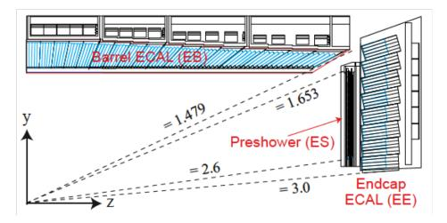
Figure 2.17: Schematic view of the ECAL.
