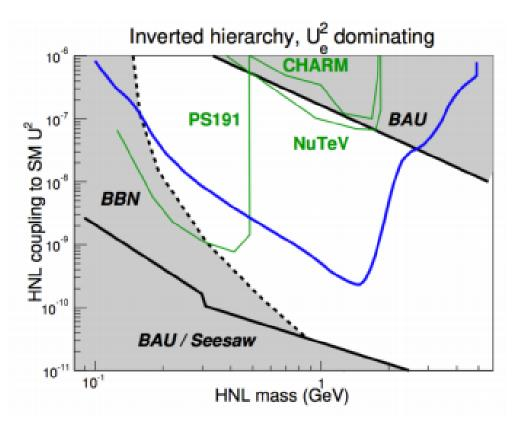
Figure 5.9: Experimental and cosmological bounds on the search for heavy neutral leptons. The exclusion limit at 90% CL SHiP could set in the case of no signal, assuming a model [185] with inverted hierarchy and a dominant electron coupling,  $U_e^2:U_\mu^2:U_\tau^2=48:1:1$ , is represented by the blue line.
