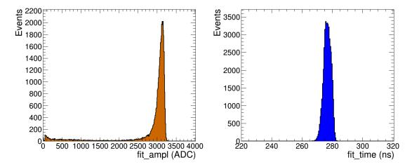
Figure 3.19: Amplitude (on the left) and time (on the right) of the crystal estimated from the template fit. The tail at low energy in the amplitude plot is due to events coming from pions present in the beam: the purity of the beam can be estimated of  $\approx 95\%$ .
