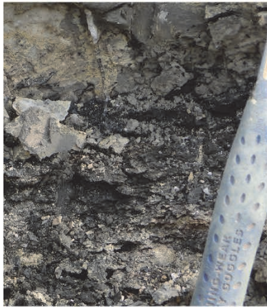
Fa5-1: Grey/black massive clay with significant amount of lignite and plant debris
