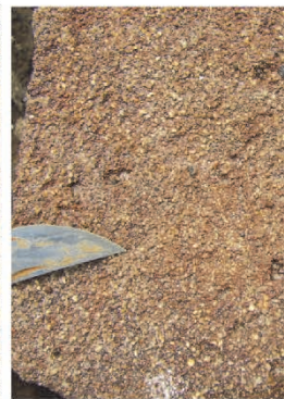
Fa3-3: Ferruginous coarse-grained sandstone
