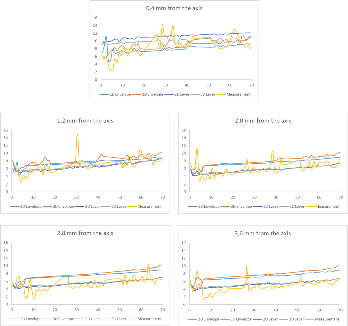
Figure 4.17 Si concentration distribution in different radial positions for all models and measurement
