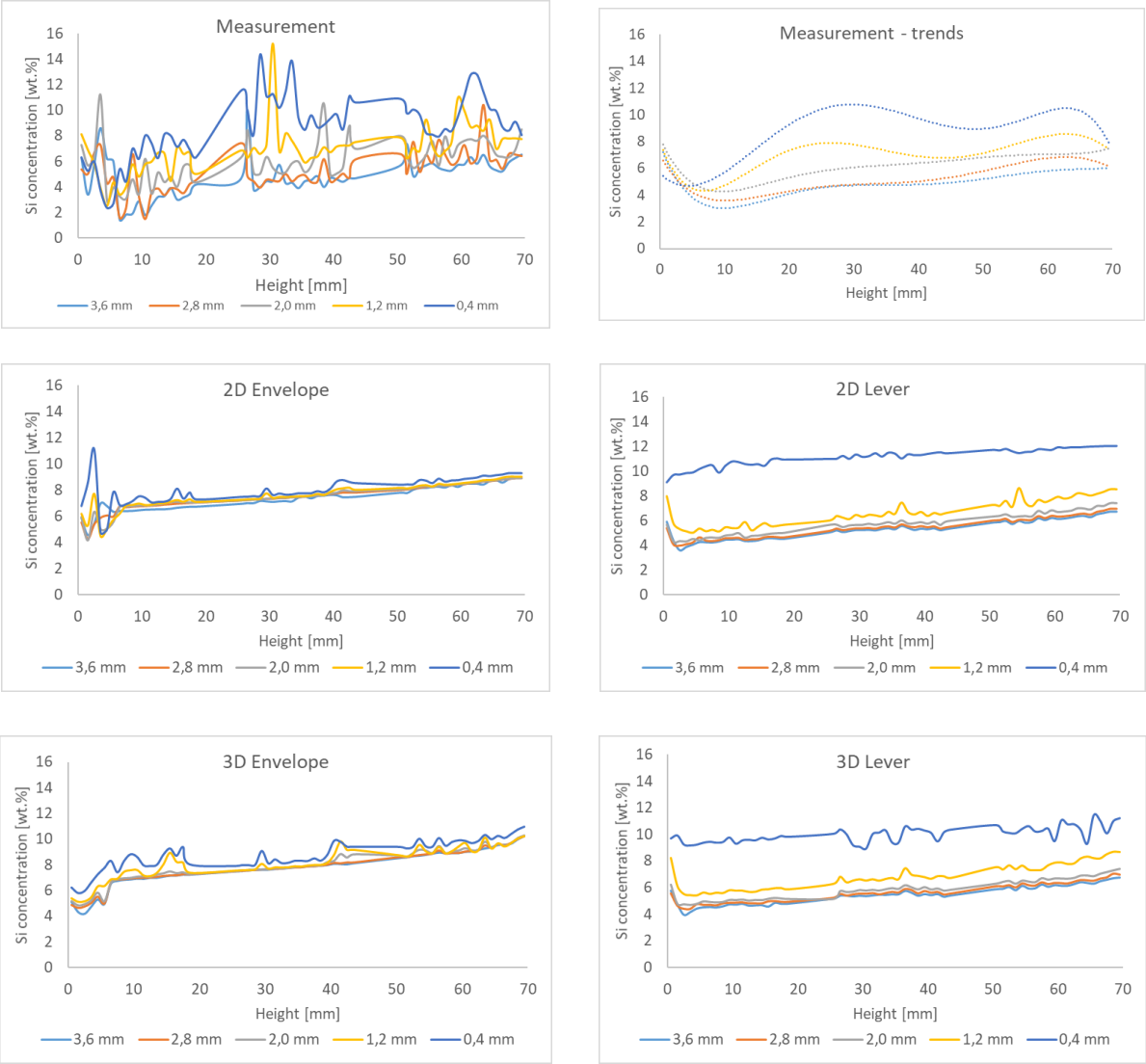
Figure 4.15 Si concentration plots based on the area avg. of the measuring windows
