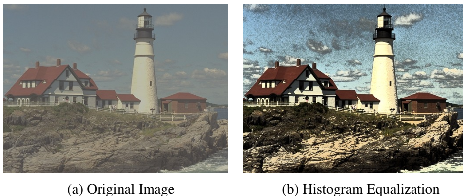
Fig. 6.1 Traditional histogram equalization for a color image. The over-enhancement problem can be observed obviously.
