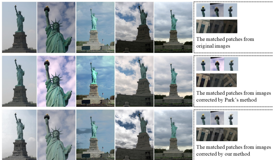
Fig. 4.6 Results on the photo collection STATUE OF LIBERTY, only five images are shown. The upper row shows the original images, the middle row shows the results by Park et al.'s method [93], the lower row shows our results.
