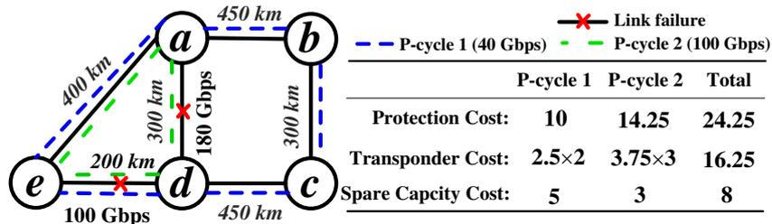
(b) Optimal solution of  $p$ -cyclesFigure 2.2: Optimal  $p$ -cycle design with the minimum CAPEX cost.
