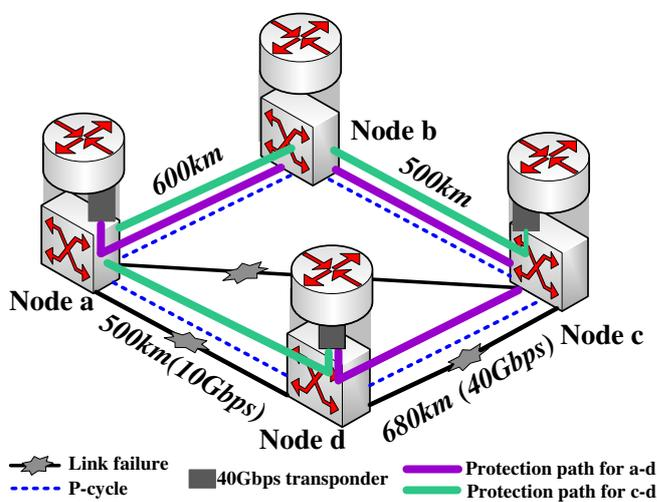
Figure 2.1:  $p$ -Cycle protection in MLR optical networks.
