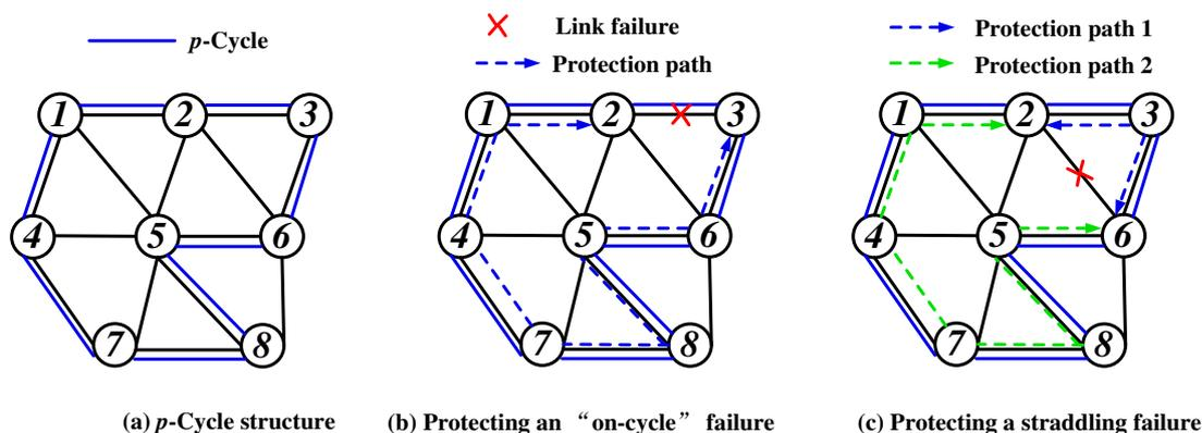
Figure 1.13: *p*-Cycle protection against single link failure.
