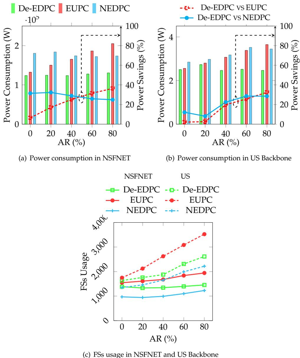
**Figure 3.9:** Power consumption and total FSs usage as a function of AR. (a) Power consumption and power savings in De-EDPC in NSFNET network. (b) Power consumption and power savings in De-EDPC in US Backbone network. (c) Total FSs usage in NSFNET and US Backbone networks.
