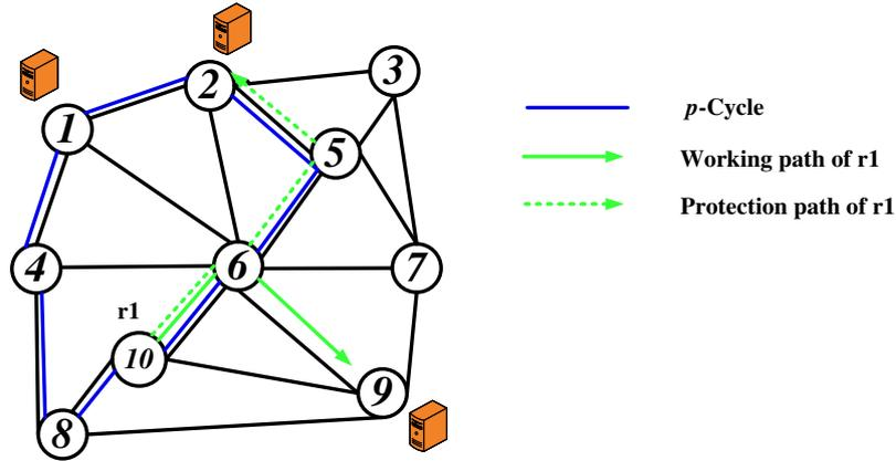
Figure 1.18: Anycast-protecting  $p$ -cycle protection scheme.
