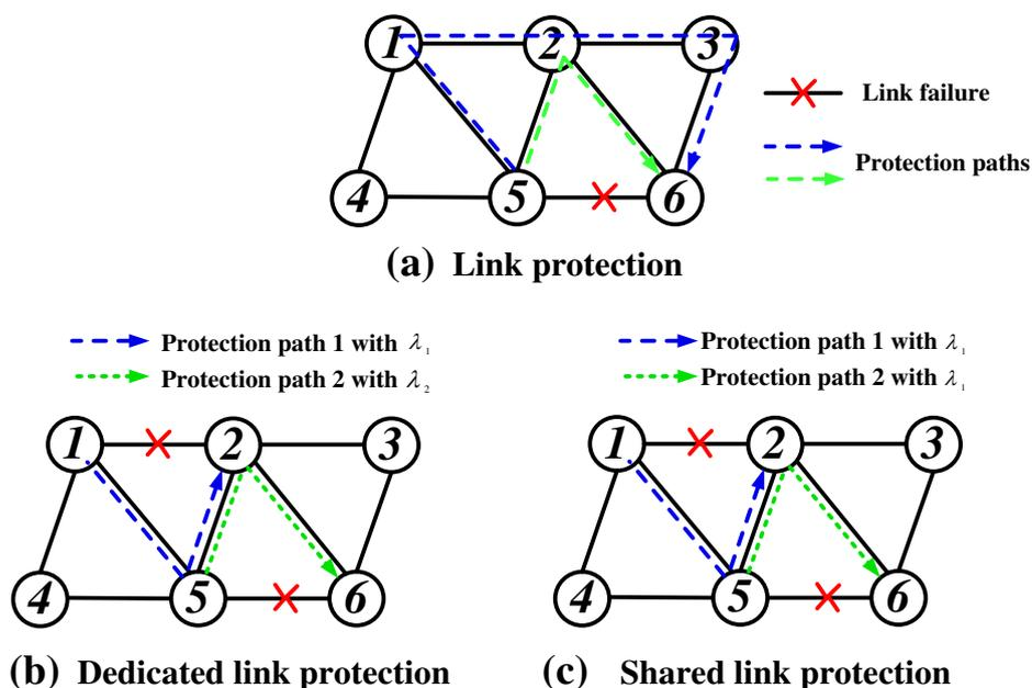
Figure 1.11: Link protection against single link failure.
