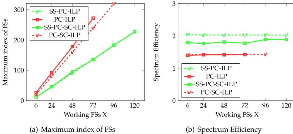
Figure 4.4: FSs allocation in COST239 topology in SS- $p$ -cycles and conventional no-shared  $p$ -cycles with/without spectrum conversion.
