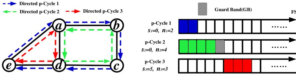
Figure 3.4: FSs allocation for different directed  $p$ -cycles.
