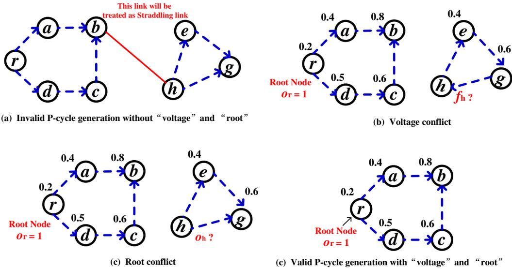
Figure 2.3: Cycle generation with and without "voltage".
