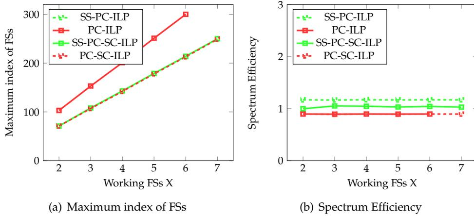
Figure 4.5: FSs allocation in US Backbone topology in SS- $p$ -cycles and conventional no-shared  $p$ -cycles with/without spectrum conversion.
