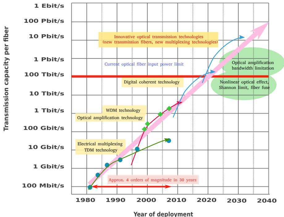
Figure 1.1: Evolution in optical transmission technology [92].
