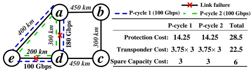
(a) Feasible solution of  $p$ -cycles
