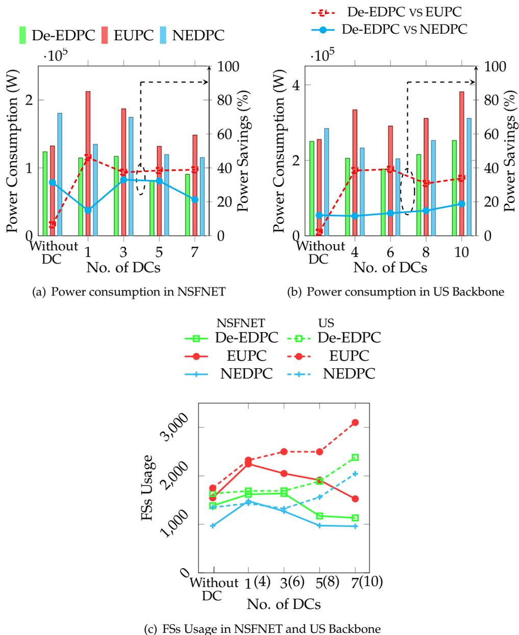
**Figure 3.10:** Power consumption and total FSs usage as a function of the number of DCs. (a) Power consumption and power savings in De-EDPC in NSFNET network. (b) Power consumption and power savings in De-EDPC in US Backbone network. (c) Total FSs usage in NSFNET and US Backbone networks.
