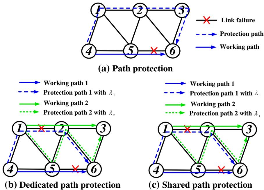
Figure 1.12: Path protection against single link failure.
