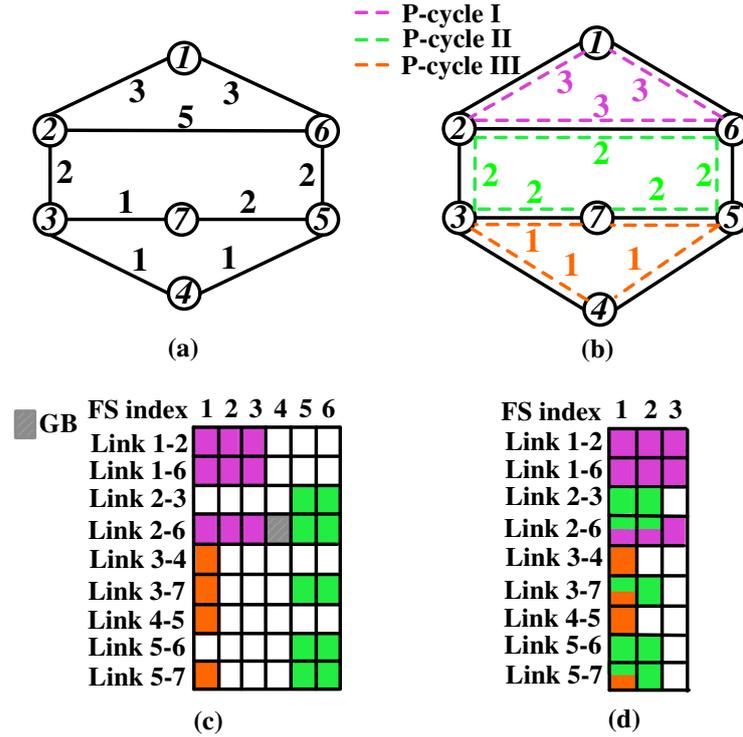
**Figure 4.1:** (a) Working FSs on each link. (b) Protection capacity in terms of FSs for each link provided by  $p$ -cycles. (c) FSs allocation in conventional  $p$ -cycles without spectrum sharing. (d) FSs allocation in SS- $p$ -cycles.
