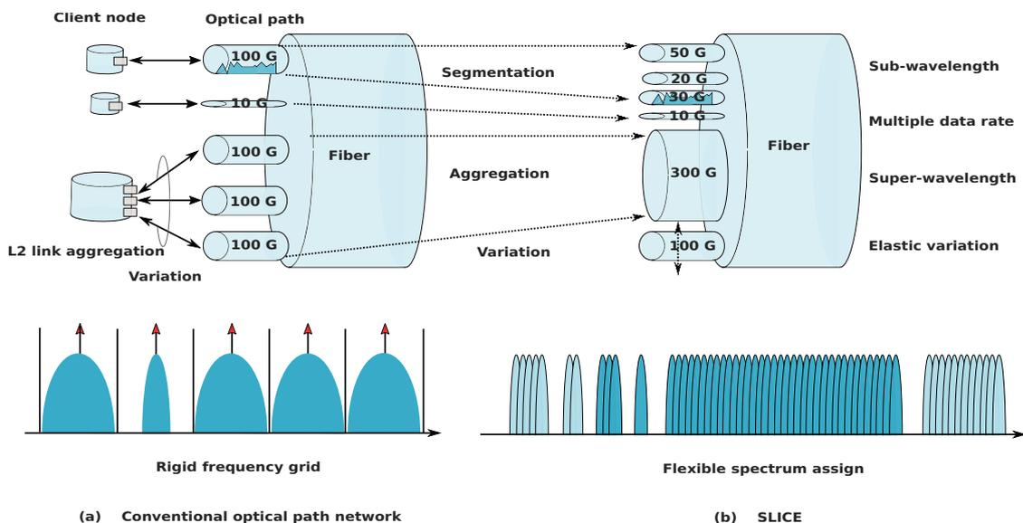
Figure 1.7: Elastic optical path provisioning [66].
