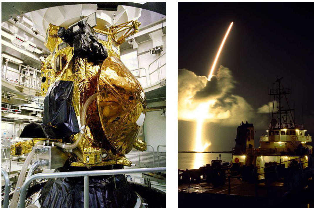
FIGURE 1.6: Left: The Cassini spacecraft with the Huygens probe to the right, atop the Titan IVB/Centaur rocket, awaiting its final shielding, weeks before launch. Credit: NASA. Right: Long exposure of the launch from Launch Pad 40, Cape Canaveral Air Station. Credit: NASA.
