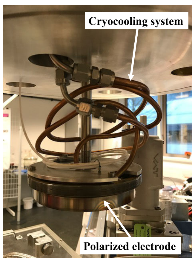
FIGURE 2.3: A close-up view of the polarized electrode montage, with the cryocooling system which consists of a soft copper pipe circulated by liquid \text{N}_2 . A solenoid valve regulates the liquid \text{N}_2 rate in order to reach the set temperature value at a \pm 1\text{K} precision. Its external and internal diameters are 6 mm and 2.5 mm, respectively. This cold trapping tube comes in contact with the electrode to trap the gas phase products. Note the gate VAT valve at the back, placed between the reactor and the mass spectrometer (MS) chamber to isolate the MS when the reactor is at atmospheric pressure.
