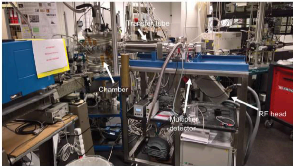
Figure B7: Experimental setup of the PAMPRE plasma reactor, coupled with a mass spectrometer (neutrals and ions).
