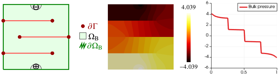
(a) Domain configuration (left), bulk pressure p (middle) and bulk pressure profile over x_1 = 0.5 (right).
