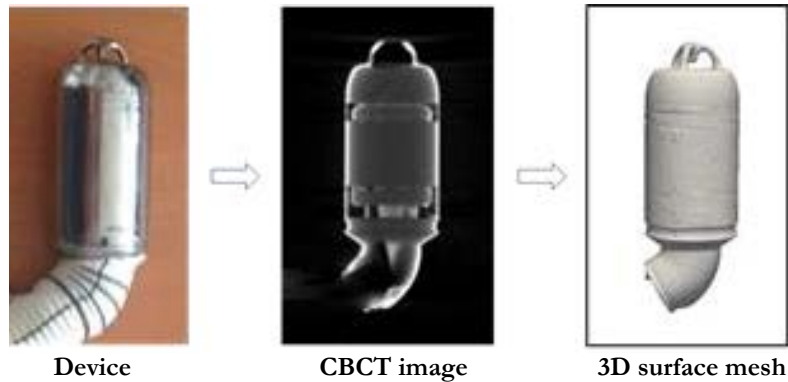
Figure 4.11 - 3D mesh of the Jarvik 2000 created from a CBCT scan with an active contour method.
