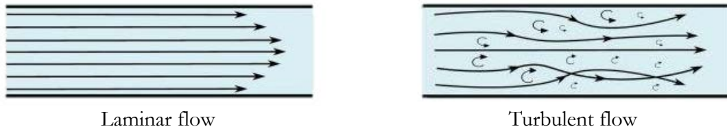
Figure 5.1 - Representation of a laminar and turbulent flow
