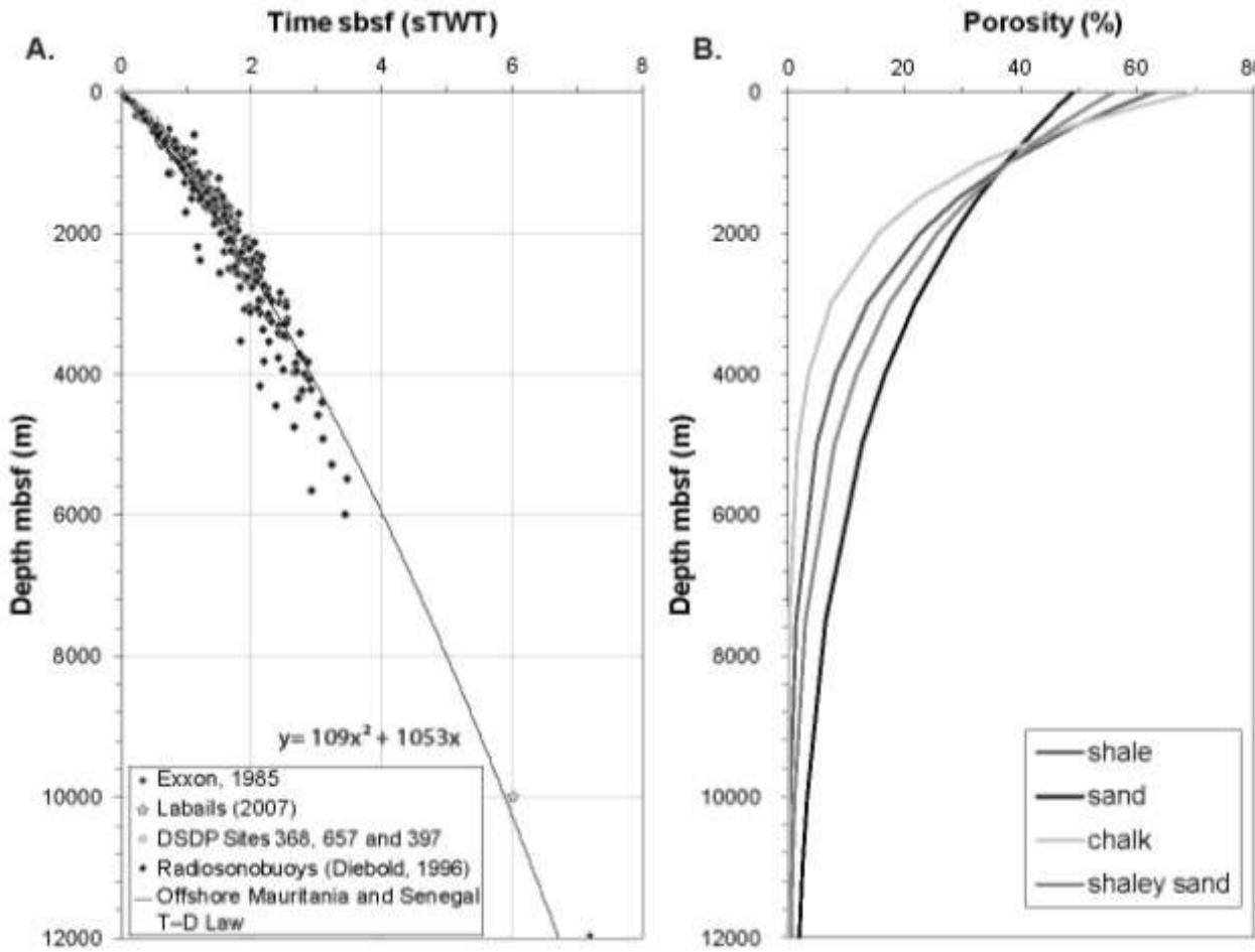
**Figure 3.4.** (A) Time–depth plot of velocity measurements from radiosonobuoys located off Mauritania and Senegal compiled by Diebold (1996) and checkshot data sourced from DSDP Sites 368, 657 and 397 initial reports (Lancelot et al., 1978b; von Rad et al., 1979; Shipboard Scientific Party, 1988). (B) Porosity curves used for decompression in FlexDecomp (Sclater and Christie, 1980).
