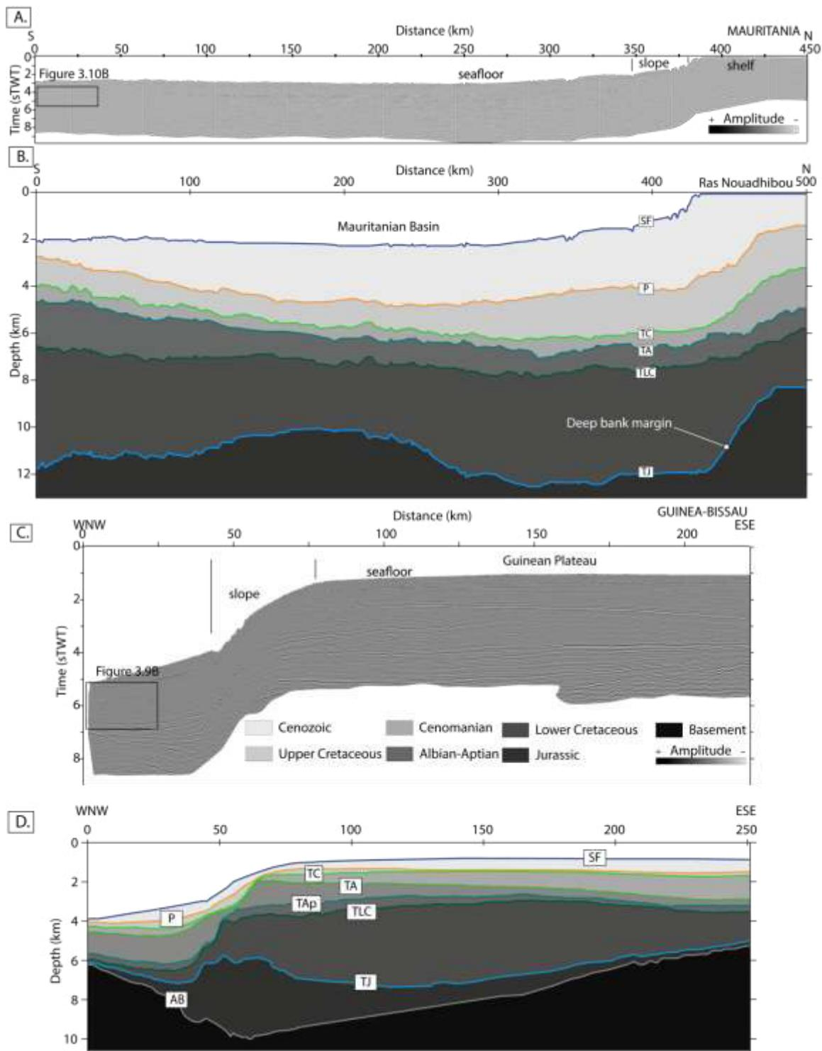
**Figure 3.7.** (A) North-South two-way time seismic section along the Mauritanian shelf (east of DSDP Site 368, offshore Mauritania), courtesy of TGS. (B) Depth-converted interpreted geological section derived from Figure 3.7A. (C) WNW-ESE two-way time seismic section through Guinean Plateau to deep-water, courtesy of TGS. (D) Depth converted interpreted geological section derived from Figure 3.7C. Legend is the same as Figure 3.6B. See Figure 3.1 for location.
