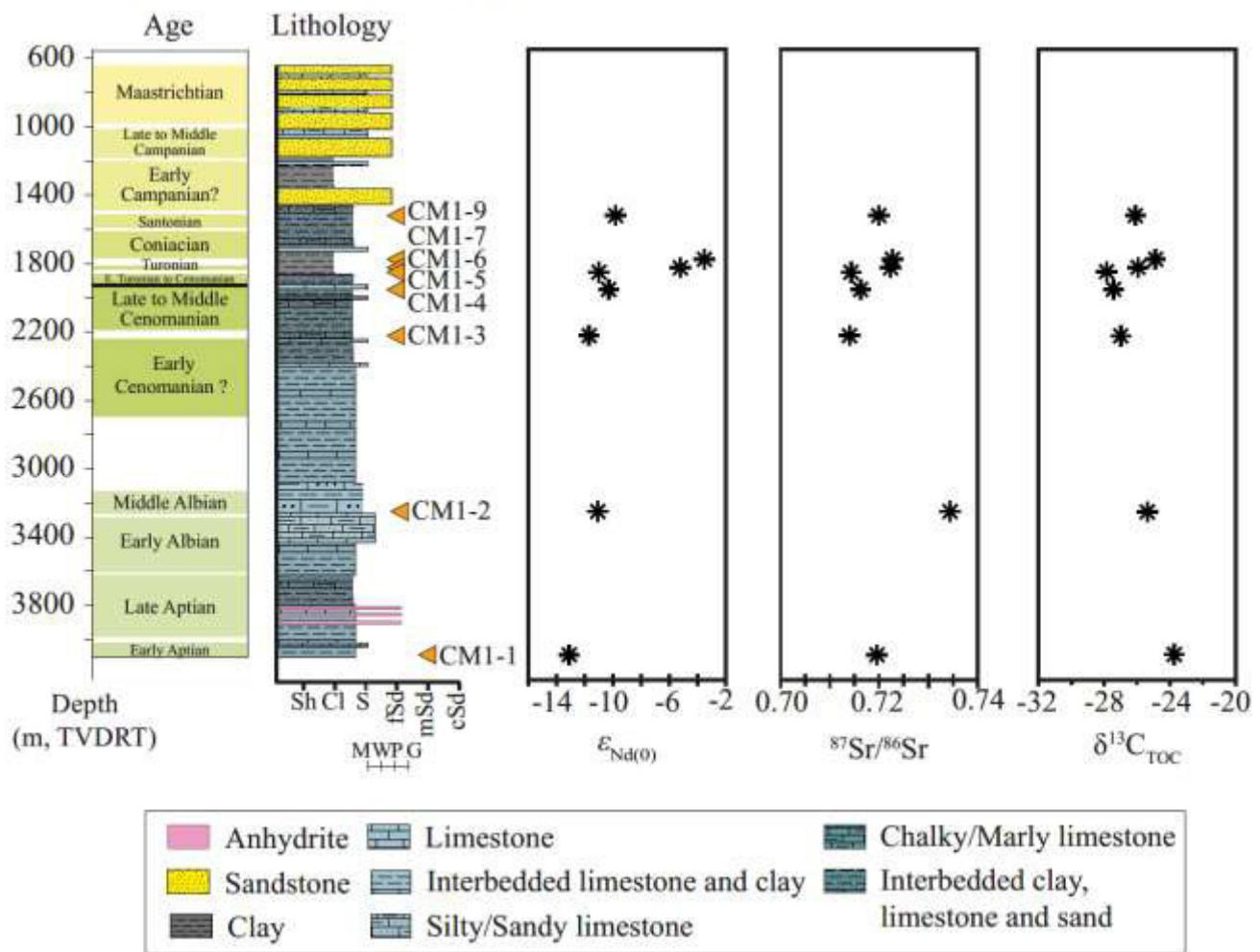
**Figure 2.3.** Stratigraphic framework, lithology,  $\epsilon_{Nd(0)}$ ,  $^{87}\text{Sr}/^{86}\text{Sr}$  and  $\delta^{13}\text{C}_{\text{TOC}}$  values of Cretaceous sediments from the CM-1 well on the Casamance continental shelf. M, mudstone. W, wackestone. P, packstone. G, grainstone. Sh, shale. Cl, clay. S, silt. fSd, fine sandstone. mSd, medium sandstone. cSd, coarse sandstone.
