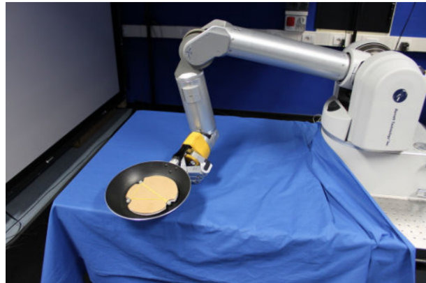
Figure 1.7 – Example of MFPS used to learn how to flip a pancake in [Kormushev et al., 2010].
