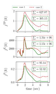
Figure 7.4 – Evolution of the total task performance cost,  $j^{\text{TP}}(k)$  (top), energy cost,  $j^{\text{E}}(k)$  (middle), and total performance cost,  $j^{\text{P}}(k)$  (bottom), for cases 1 and 2.
