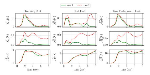
Figure 7.3 – Time evolution of the tracking,  $j_i^{\text{TP}}(k)$ , goal,  $j_i^{\text{TP}}(k)$ , and task performance,  $j_i^{\text{TP}}(k)$ , costs for each task in the example problem from Sec. 6.6. The costs are calculated as the area under the curves, but looking at their evolution allows the task performance to be analyzed.
