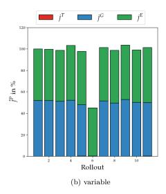
Figure 9.7 – Evolution of the performance cost in percentage using static, (a), and variable, (b) weights (deterministic and stochastic policies). Each rollout cost is broken up into the component tracking,  $j^{\rm T}$ , goal,  $j^{\rm G}$ , and energy,  $j^{\rm E}$ , costs.
