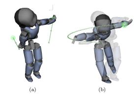
Figure 1.2 – Incompatible and infeasible tasks which result in (a) the robot getting stuck in a constrained configuration and (b) a loss of equilibrium.
