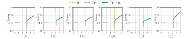
Figure 6.11 – The evolution of the inequality constraints for the lower joint position limits for case 3, evaluated at the prioritized optimum,  $\chi^*$ . The  $G\chi^*$  line is darkened where the prioritized optimum would violate the constraint. A violation indicates that the prioritized optimum is infeasible and thus activates certain constraints in the QP.
