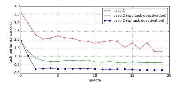
Figure 8.3 – Cost curves for the TCFM optimizations for both test cases. Note that each update corresponds to 15 policy rollouts. For all cases, the TCFM, using DMPs and PI<sup>BB</sup>, is stopped after 300 rollouts, because the update policy convergence criterion is never attained.
