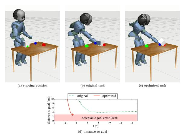
Figure 9.6 – This figure shows the original and optimized tasks for the "Moving a Heavy Weight" simulation detailed in Sec. 9.3.2. (a) shows the initial starting posture. In (c), it can be seen that the robot comes up just short of its goal location. By optimizing the middle waypoint of the task, the robot is able to accelerate more at the beginning of the movement, building up sufficient inertia to reach its goal within the acceptable error, as demonstrated by (d).
