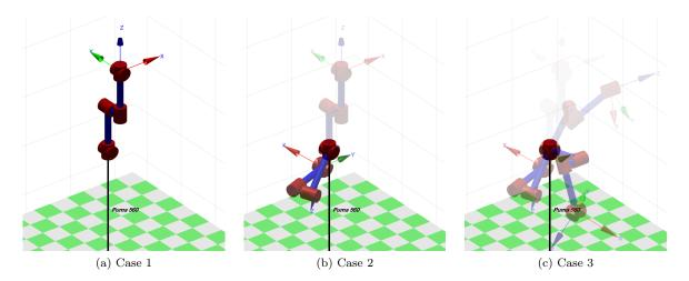
Figure 6.7 – The robot motions for the three task feasibility cases. In case 1, the robot maintains its initial feasible posture. In case 2, the reference posture is set immediately to  $q_{\rm IF}$ , an infeasible posture, and the robot moves quickly to the reference. In case 3, a joint-space task trajectory is used to move the robot more gradually to  $q_{\rm IF}$ .
