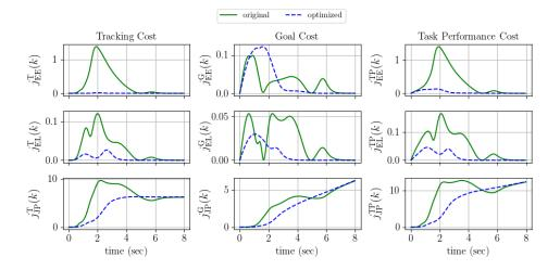
Figure 7.11 – Time evolution of the tracking,  $j_i^{\text{TP}}(k)$ , goal,  $j_i^{\text{TP}}(k)$ , and task performance,  $j_i^{\text{TP}}(k)$ , costs for each task in the example problem from Sec. 6.6 is used. The costs are calculated as the area under the curves, but looking at their evolution allows the task performance to be analyzed.
