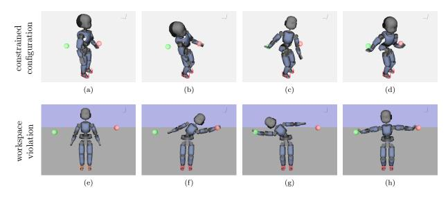
Figure 8.1 – (a) - (d) show the constrained configuration scenario and (e) - (h) show the workspace violation scenario. (a) & (e) starting positions. (b) & (f) left hand + standing tasks end configurations. (c) & (g) right hand + standing tasks end configurations. (d) & (h) end configurations of left hand, right hand and standing task combinations where the robot cannot attain both goal positions (spheres) simultaneously.
