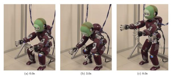
Figure 1.10 – In (a), (b), and (c), a time-lapse is shown of an optimized standing motion performed by an iCub robot, which was found using the task compatibility and feasibility maximization algorithm developed in this work. The un-optimized motion caused the robot to fall.
