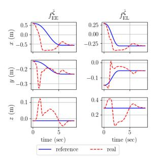
Figure 6.14 – Task reference and real position values throughout the movement. As can be seen, the trajectory tracking suffers in the middle of the movement, which indicates some decrease in task compatibility/feasibility.
