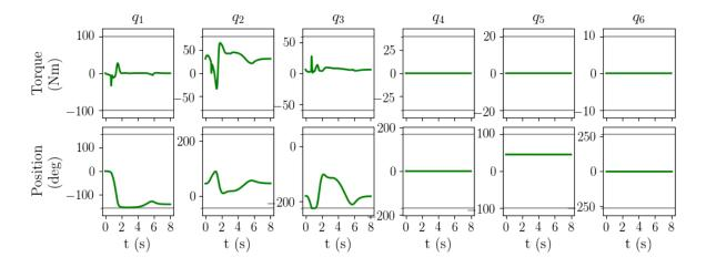
Figure 6.15 – The evolution of the joint torques and positions for the temporal example. During the movement,  $q_1$  and  $q_3$  hit their lower position limits, thus indicating an infeasibility.
