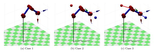
Figure 6.1 – The three task compatibility cases. The desired positions for the EE and elbow tasks are shown by the blue and red spheres respectively. For case 1, the starting positions are the same as the goal positions so they are not shown. For case 3, trajectories are used and shown by the blue and red lines.
