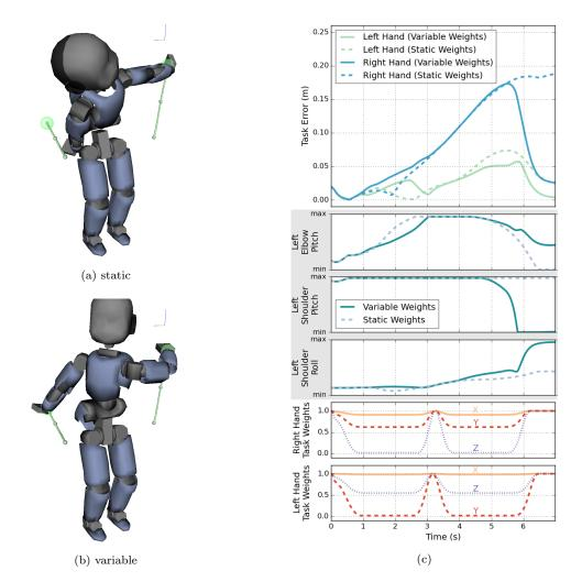
Figure 9.1 – The constrained configuration scenario. (a) and (b) show the task combination results using static and variable weights respectively. (c) plots provide the simultaneous evolution of various task parameters.
