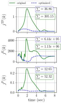
Figure 7.12 – Evolution of the total task performance cost,  $j^{\text{TP}}(k)$  (top), energy cost,  $j^{\text{E}}(k)$  (middle), and total performance cost,  $j^{\text{P}}(k)$  (bottom), for original and optimized policies.
