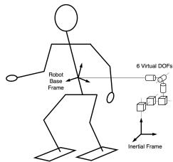
Figure 2.1 – A diagram indicating visually what it means to include the root link pose in the parameterization. The 6-DoF of the floating base are modeled as a 6-DoF linkage with the world or inertial frame. Image taken from [Mistry et al., 2010].
