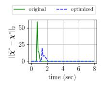
Figure 7.15 – Distance between the prioritized optimum,  $\chi^*$ , and the controller optimum,  $\tilde{\chi}^*$ , for the original and optimized policies. Any nonzero distance means the prioritized optimum violates the inequality constraints.
