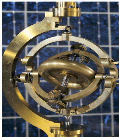
Figure 1.1 A model of the gyroscope built by Foucault in 1852 (Credits: Musée des Arts et Métiers, Paris).
