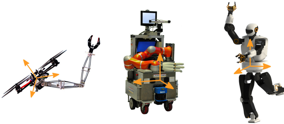
Figure 7.4: Three different multi-joint mobile robots at LAAS: the flying manipulator Aeroarm (left), the mobile manipulator Jido (center), and the humanoid robot Talos (right). The usual choices for their root frame placement are displayed.
