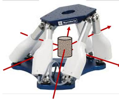
Figure 10.4: Hexapod testing machine that could be positioned *in-situ*. The three red arrows indicate the possible acquisition windows where the beam is not masked by the 6 actuators.
