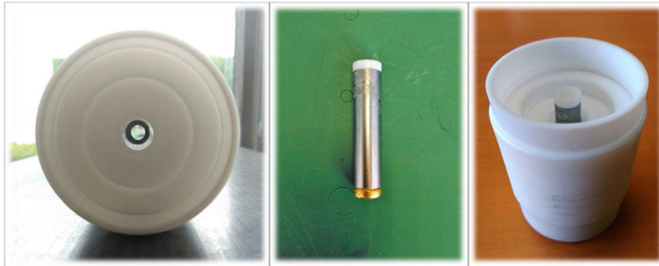
Figure A.3 – The Teflon container is drilled along the central axis (left). An aluminum cylinder with a Teflon layer at the top and a screw nut at the bottom (center). By pushing the aluminum cylinder with a screw, the PMMA support and the fiber bundle can be easily separated after gluing (right).
