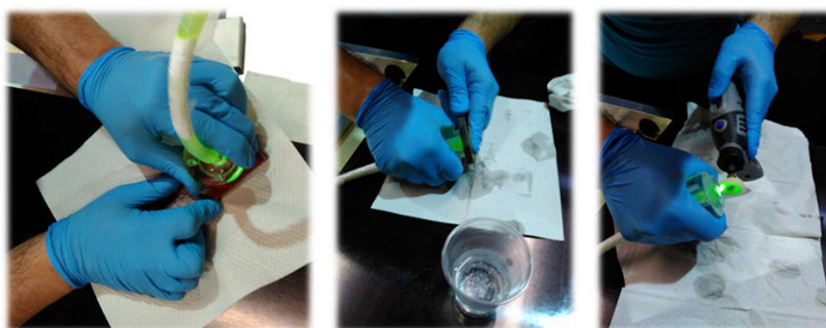
Figure A.6 – We polish off the protruding 5mm-long fibers with heavy-grade sandpapers (200, 320 grit) (left). Then we polish the fiber ends and PMMA surface with fine-grade sandpaper (800, 1200 grit) (center) and buff the fiber ends with a 1-inch loose cotton wheel on an electric polisher rotating at a spindle speed below 10000 revolutions per minute (right).
