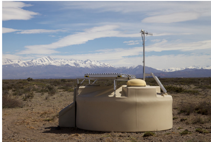
Figure 3.6 – Water-Cherenkov detector with a scintillator detector on top.
