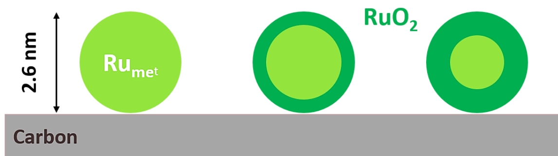
Figure 44. Sketch of the models used for photoemission spectra simulation with the SESSA software. Panel A: “layered sphere” morphology, metallic ruthenium particles ( d = 2 nm) covered by \text{RuO}_2 shell of various thickness.
