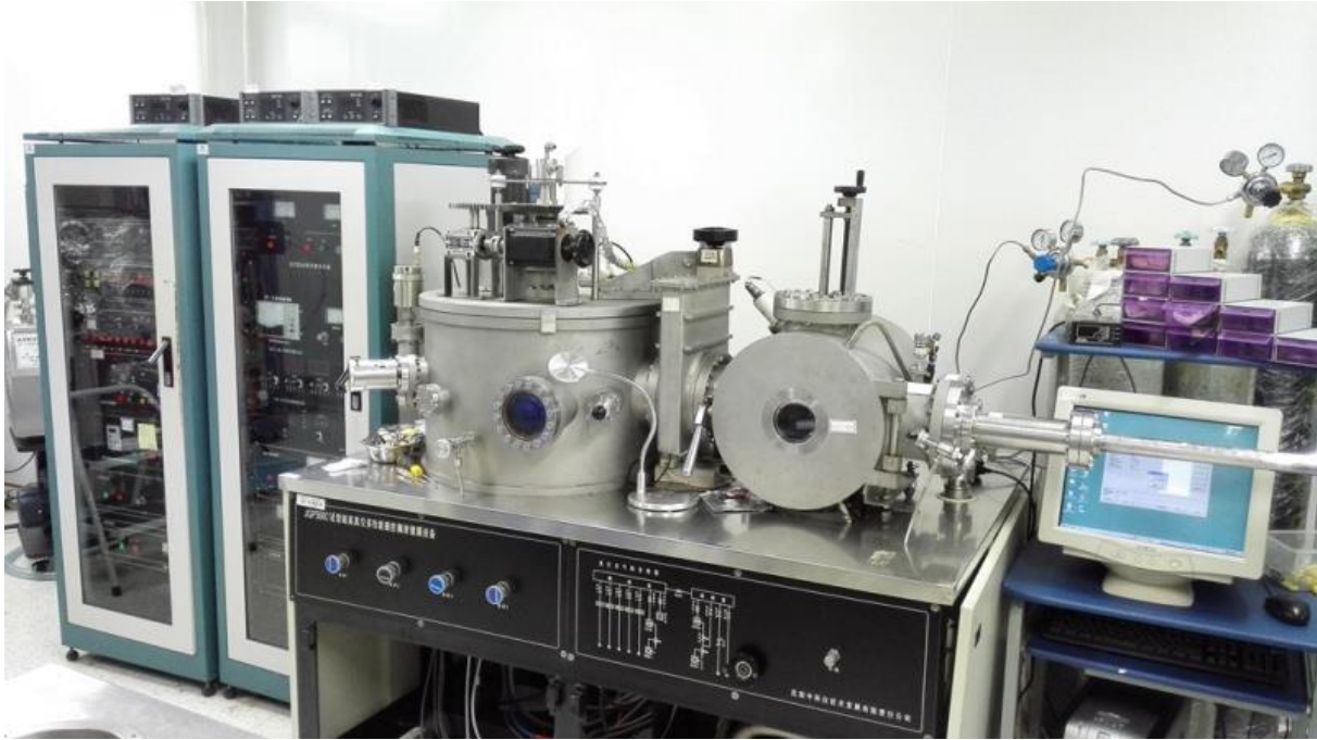
Figure 1.7: Magnetron sputtering setup of Institute of Precision Optical Engineering of Tongji University in China.
