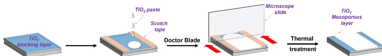
Figure II-10: Schematic representation of doctor-blade technique on TiO 2 (blocking layer)/FTO substrate.
