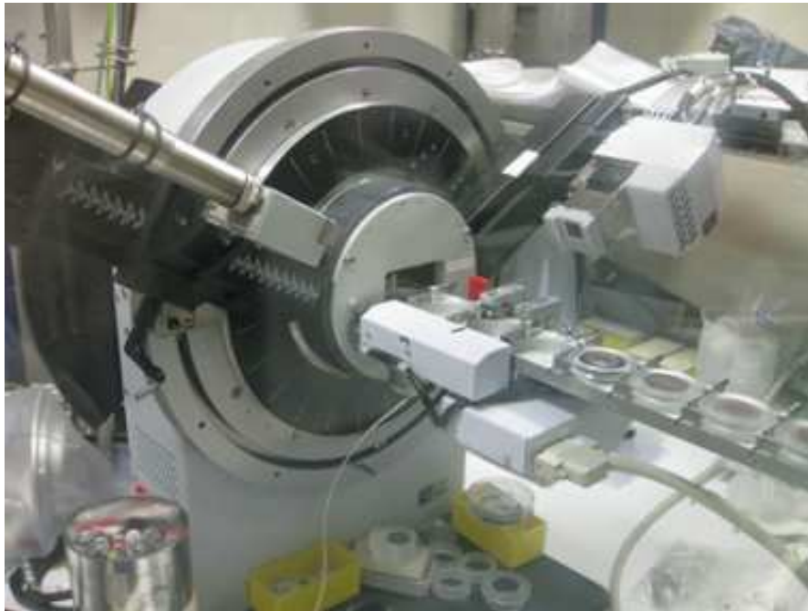
Figure 3.15 – X-ray diffractometer Bruker D8 Advance, in Bragg-Bentano configuration and Ge-primary monochromator.
