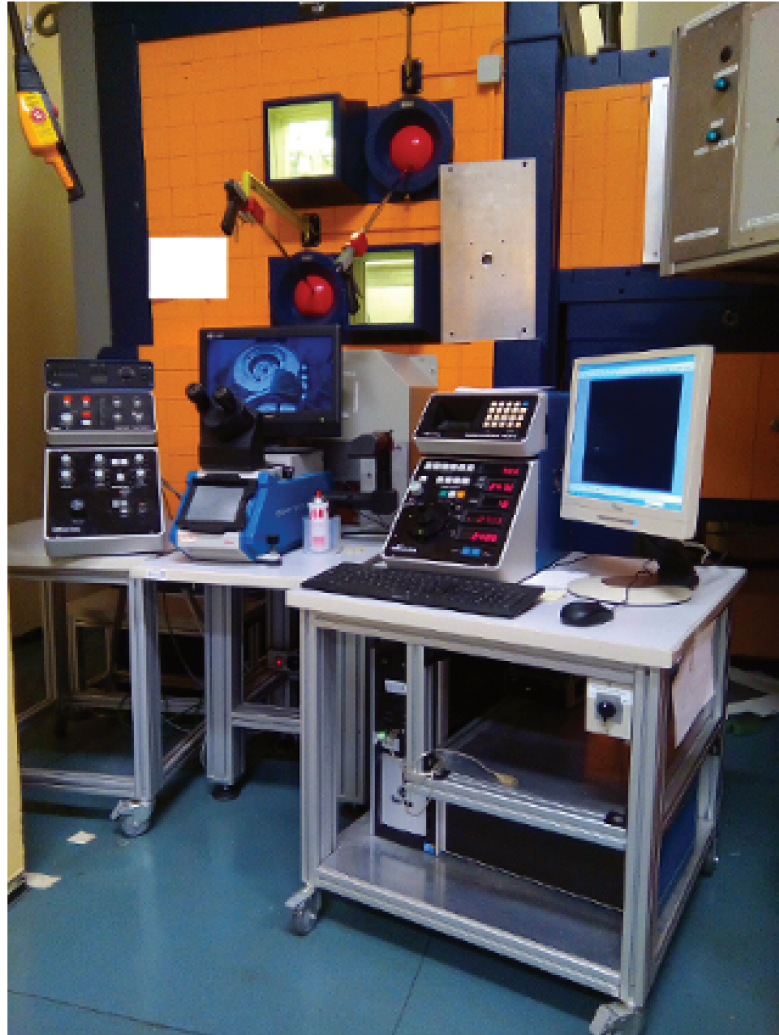
Figure 3.14 – Shielded optical microscope (LEICA Telatom 3) equipped with a Micro-Duomat 4000E microhardness Vickers tester
