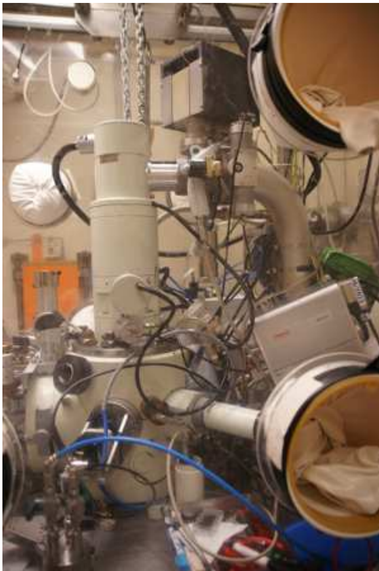
Figure 3.16 – Scanning electron microscope in glove box.
