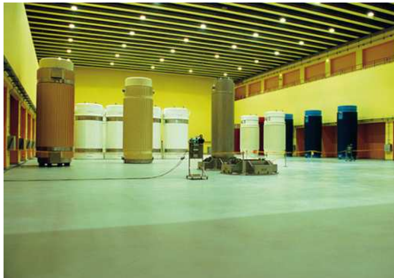
Figure 1.23 – Dry storage: casks at the ZWILAG facility in Switzerland [51].
