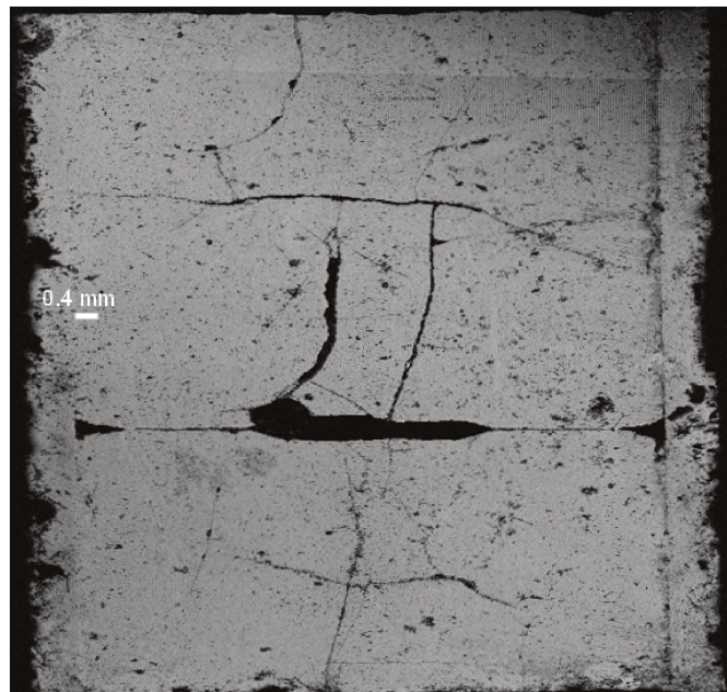
Figure 4.11 – Acoustic image of the longitudinal section of the investigated pellet, acquired at 140 MHz, 15 \mu\text{m} below the surface.
