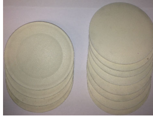
Figure 3.15: Manufactured sub-lenses for the (left side) smooth[2\pi] and (right side) smooth cases after being pressed.
