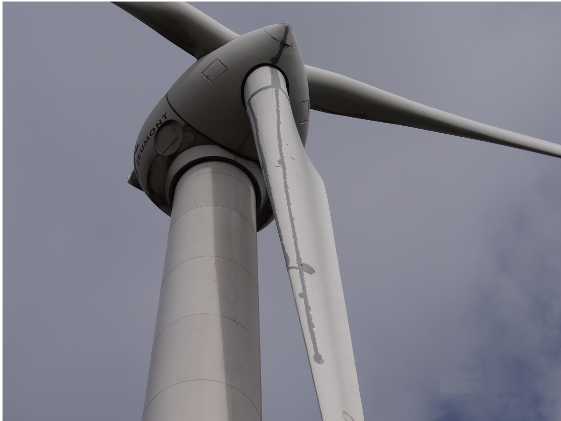
Figure 4.11: Photo of the pressure side of the wind blade after installation of sensors
