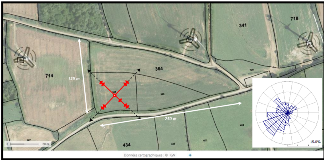
Figure 4.7: Final position of the met mast and wind rose of the area.
