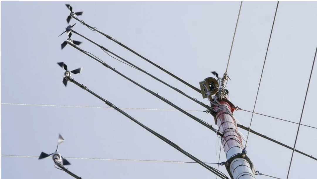
Figure 4.9: Photo of the sensors on the met mast
