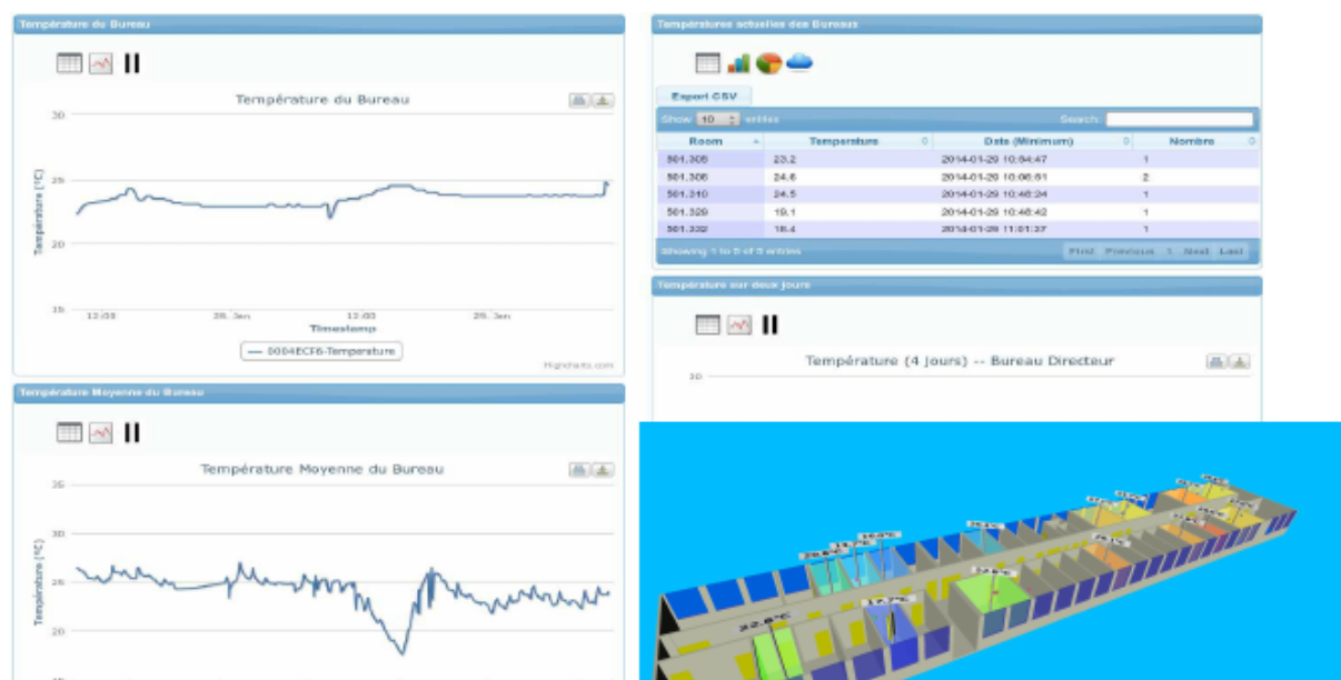
Fig. 5.7 SoCQ4Home DashBoard and 3D projection of sensor devices [160].
