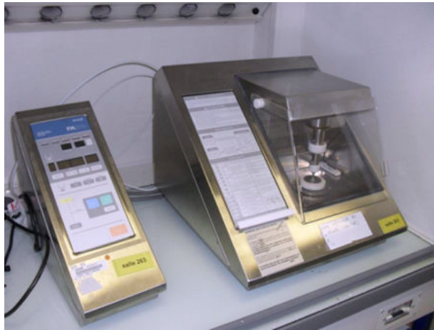
FIGURE 1.29 – Hamamatsu PA103 Automated Decapsulation Machine
