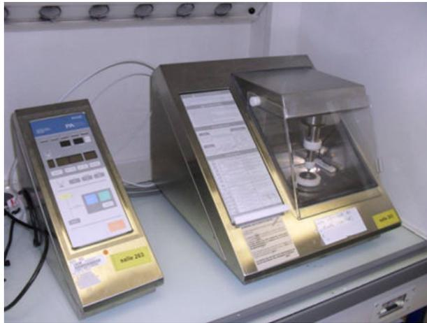
FIGURE 1.29 – Hamamatsu PA103 Automated Decapsulation Machine
