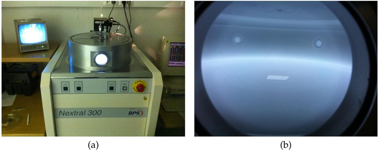
FIGURE 1.33 – A plasma etching machine (a) and a sample being processed(b)
