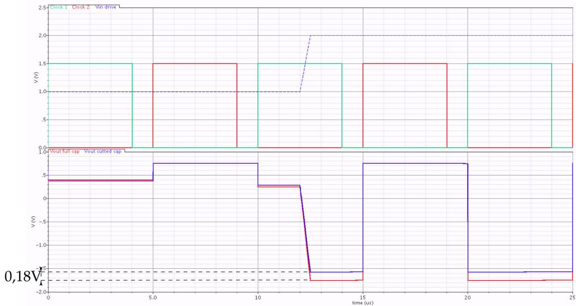
FIGURE 6.9 – Voltage values outputted by the switch-capacitor amplifier for full and cut fringe capacitor
