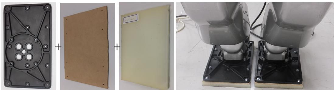
Figure 3.8 Photo of HRP-2's feet with flexible soles
