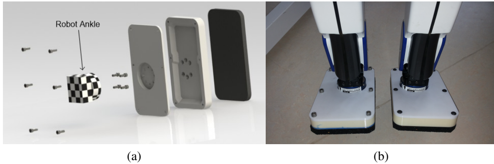
Figure 5.9 (a): new HRP-4's feet; (b): photo of HRP-4's feet with soft soles
