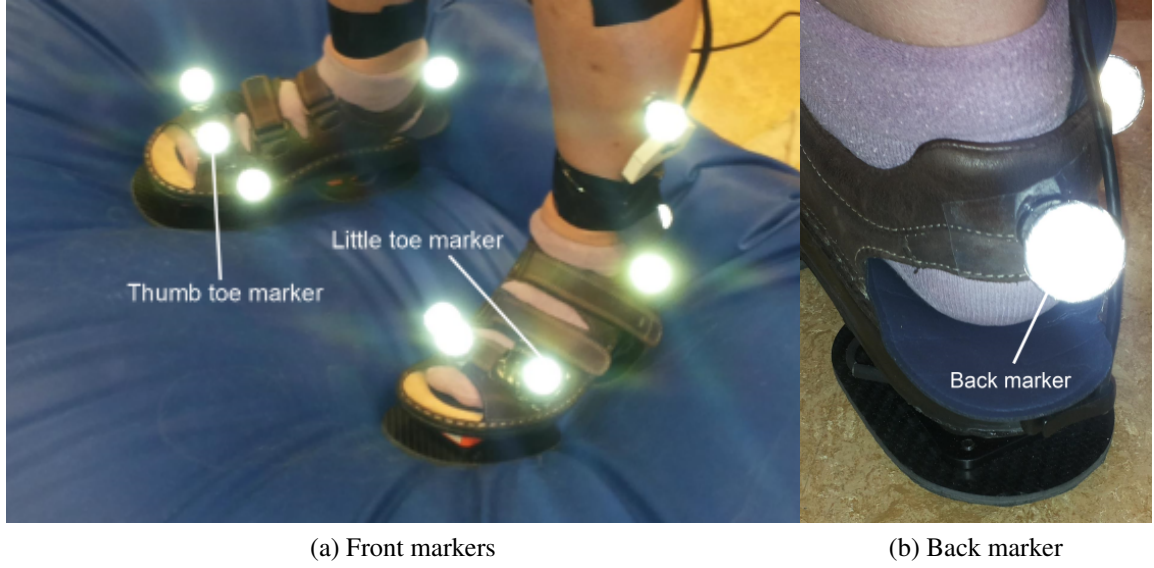
Figure 2.4 VICON markers on ForceShoes
