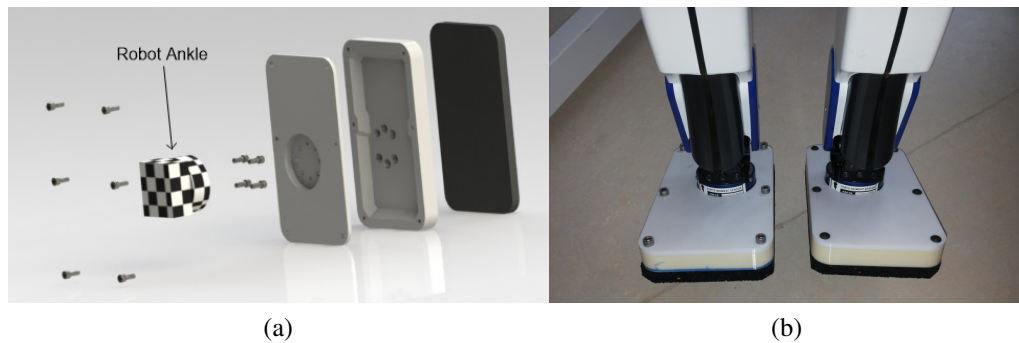
Figure 4.6 (a): new HRP-4's feet; (b): photo of HRP-4's feet with flexible soles
