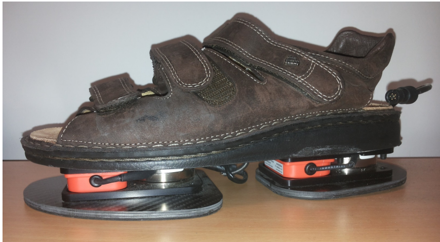
Figure 2.3 ForceShoe system; MTx (orange boxes); F/T sensors (steel grey cylinder)
