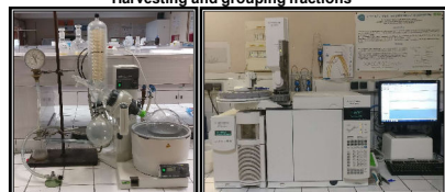
Rotary evaporator Quantification by GCMS and weighing
