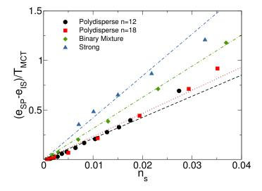
**Figure 4.14** – Difference in energy between saddles and corresponding minima as a function of the saddle index for four different models. The *y*-axis is rescaled by  $T_{MCT}$  to compare. Linear fits are performed in regions accessible by standard simulations.
