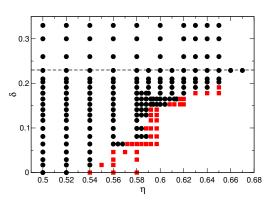
(b) Phase diagram of polydisperse soft-sphere in our swap simulations. The softness parameter is n = 36 which makes the system close to a hard sphere system. On the *x*-axis we plot the packing fraction and on the *y*-axis the polydispersity. Black circles indicate stable fluid phase and red squares indicate presence of order and long-range density fluctuations.
