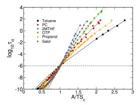
(a) Adam-Gibbs plot of common logarithm of relaxation times as a function of inverse configurational entropy times temperatures for experimental data. Only 2MTHF shows a linear agreement with the Standard Adam Gibbs relation. Lines are from fit of the Generalized Adam Gibbs performed at experimental timescales.
