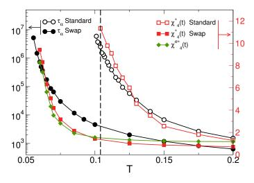
**Figure 3.18** – Temperature evolution of dynamic susceptibilities (right axis) and relaxation times (left axis), the vertical dashed line is  $T_{MCT} = 0.104$ . Whereas  $\chi_4^d(t)$  grows together with  $\tau_{\alpha}$  in standard simulations,  $\chi_4^d(t)$  and  $\chi_4^{\sigma}(t)$  behave similarly and have a very different temperature dependence which mirrors instead the evolution of the swap relaxation time.
