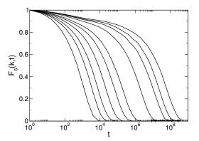
(b) Self-intermediate scattering function for swap simulations of the N=3000 system. No short time relaxation is present and the decrease of temperature has the main effect of stretch times for short ranged vibrations. Results are T=0.200, 0.120, 0.092, 0.070, 0.0555, 0.047, 0.035, 0.030, 0.028, 0.026.
