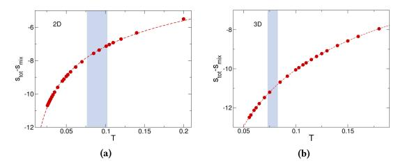
**Figure 4.2** –  $s_{\text{tot}} - s_{\text{mix}}$  as a function of T. The dashed curve is the Rosenfeld-Tarazona expression: (a)  $s_{\text{tot}} - s_{\text{mix}} + 2 \ln \Lambda \propto T^{-2/7}$ , (b)  $s_{\text{tot}} - s_{\text{mix}} + 3 \ln \Lambda \propto T^{-2/5}$ . Shaded areas indicate the location of the laboratory glass transition.
