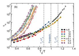
(b) Relaxation times obtained from standard (open symbols) and swap (filled symbols) dynamics for various size polydisperse models of various softness (n) and non-additivity ( $\epsilon$ ) are shown in an Arrhenius form with rescaled temperature  $T_g/T$ , where  $T_g$  is estimated as in (a). For all models the thermalization speedup near  $T_g$  is of about 10 orders of magnitude, some models being structurally stable down to temperatures below  $T_g$ .
