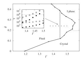
(a) Phase diagram of polydisperse softspheres obtained with swap simulations taken from Ref. [79]. The softness parameter is n = 12. On *x*-axis the thermodynamic parameter  $\Gamma = \rho T^{-1/4}$ . On the *y*-axis the particle polydispersity  $\delta$ . Authors identified three phases: a high temperature fluid, a crystal, and a inhomogeneous solid I. The vertical line in the fluid phase represent the kinetic glass transition.
