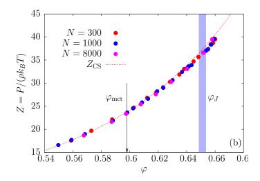
**Figure 4.1** – Equilibrium equation of state obtained with swap simulations of continuously polydisperse hard spheres for different system sizes. Our equilibrium data go beyond the shaded area, which represents the determined range of jamming densities. The dashed line is the Carnahan-Stirling empirical expression [184].
