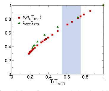
**Figure 4.6** – Red squares indicate configurational entropy by thermodynamic integration. Green triangles indicate the inverse of the point-to-set length normalized by its value at the Mode-Coupling temperature  $\xi_{MCT} = 2.57$ . The shaded area indicate the location of the laboratory glass transition.
