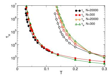
**Figure 3.25** – Relaxation time as a function of the temperature for standard (empty symbols) and swap (full symbols) simulations for two system sizes N=300, N=20000. In standard simulations density relaxations decouples for different system sizes whereas orientational degrees of freedom have same relaxation timescales. In swap simulations orientational and translational relaxation have the same timescales to happen and smaller size effects are observed.
