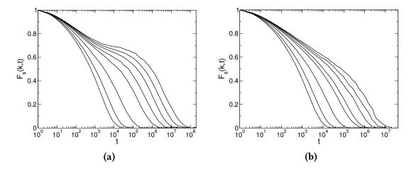
**Figure 3.23** – Self-density relaxation times for standard Monte Carlo simulations in two dimensions for a system of N=300 (a) and N=20000 (b) particles. We notice the absence of well defined plateau increasing the system size. The results are obtained at T=0.300, 0.250, 0.200, 0.0.170, 0.160, 0.150, 0.145, 0.140.
