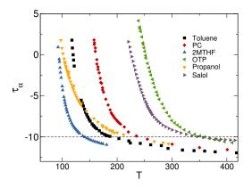
(a) Relaxation times from dielectric spectroscopy and dynamic light scattering for six molecular glass formers. Data for Toluene, PC, OTP, Salol are taken from Ref. [211], for Propanol and 2MTHF are from Ref. [133].
