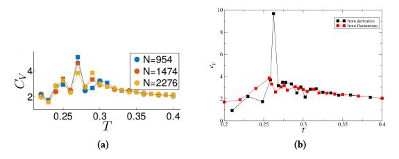
**Figure 3.6** – Specific heat of swap simulations computed both using derivatives  $c_V = \partial \langle U \rangle / \partial T$  (squares) and standard deviations  $c_V = (\langle U^2 \rangle - \langle U \rangle^2)/kT^2$  (circles) of the potential energy. (a) results are reproduced from Ref. [80]. (b) equivalent results obtained in our simulations. The peak in our case is more evident and coincide with phase separation in the system.
