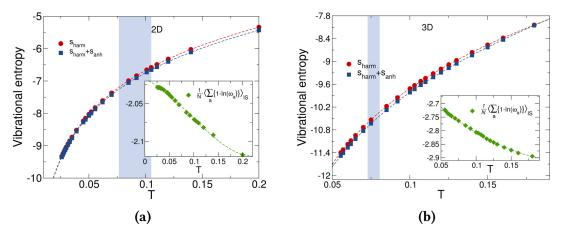
**Figure 4.4** – The harmonic vibrational entropy  $s_{\text{harm}}$  and anharmonic correction  $s_{\text{anh}}$ . The dashed curves are obtained by a quadratic fit for  $(1/N) \sum_{a=1}^{3N} \{1 - \ln(\omega_a)\}$ . (a) 2D system, (b) 3D system. Shaded areas indicate the location of the laboratory glass transition.
