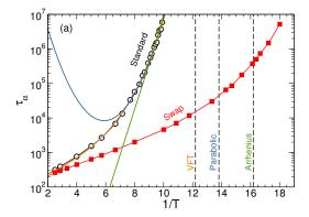
(a) Relaxation times for the non-additive model with n = 12 and  $\epsilon = 0.2$  for standard and swap Monte Carlo dynamics. The standard dynamics is fitted with the VFT, parabolic and Arrhenius laws, as shown with lines, which are used to estimate the location of the experimental glass temperature  $T_g$ , as shown with vertical dashed lines. For this system, the swap dynamics is able to provide stable and thermalized configurations at temperature below  $T_g$ .
