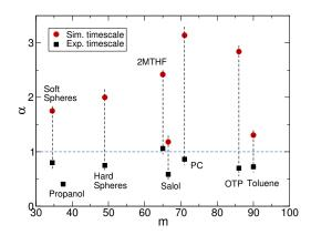
(b) Value of the coefficient  $\alpha$  from the GAG equation (Eq. 4.20) for six experimental and two computational glass-forming liquids as a function of the fragility parameter m both in experimental and computational timescales.
