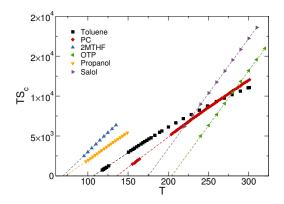
**(b)** Configurational entropy times temperature plotted as a function of temperature from calorimetric measurements. Data for Toluene and PC are from Ref. [212], for Propanol, 2MTHF, OTP, Salol are from Ref. [133].
