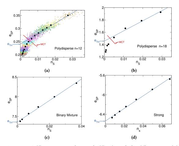
**Figure 4.12** – Saddle energy  $e_{SP}$  as a function of saddle index  $n_S$  for four different supercooled liquids: (a) polydisperse non-additive model with n=12, (b) polydisperse additive model with n=18, (c) binary mixture, (d) strong glass-former. Straight lines are fits on the standard simulations region, arrows roughly indicate the correspondent location of the Mode-Coupling. Figure (a) include also the scatter plot of the data, different colors are for different sampling temperatures.
