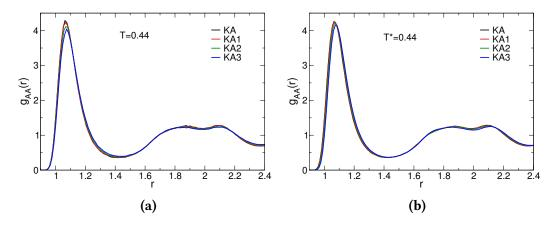
**Figure 3.22** – The radial distribution function for the particles in the species A in four models. KA indicates the original binary mixture. KA1, KA2, KA3 indicate the three modified systems. (a) results are given for temperature T = 0.44. (b) results are given for the rescaled temperature  $T^* = 0.44$ .
