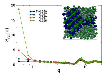
**Figure 3.7** – Partial structure factor  $S_{CC}(q)$  for small particles in the ternary mixture. It is featureless at high enough temperatures, T = 0.350, displays strong composition fluctuations at low q in the fluid at T = 0.267, that may eventually lead to a demixed state at long times. For  $T \leq 0.26$ , the system is demixed, as shown for T = 0.256. The inset shows a representative snapshot of a demixed and partially crystallized system at T = 0.256.
