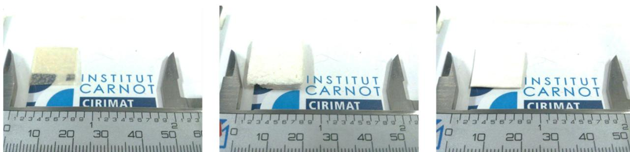
Fig. 1. The three different materials: (left) a hot air dried Xero, (middle) a freeze dried Lyoph, and (right) a supercritical dried sample SCC.
