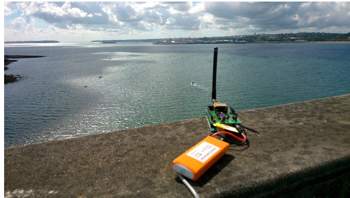
Figure 4.4 – LoRa emitter is placed on the Elorn bridge in our experimental measurement at Plougastel.
