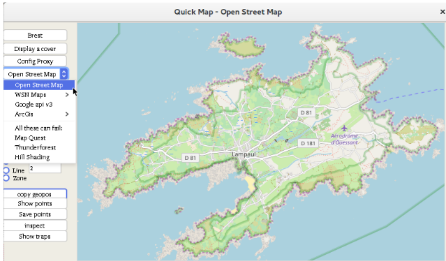
Figure 3.2 – QuickMap: a map browser allows to select various kind of tile server for retrieving tile map for free GIS database such as OpenStreetMap. In this figure, QuickMap is used to select a area at Ouessant island (15.58 km 2 ) in Brittany, France.
