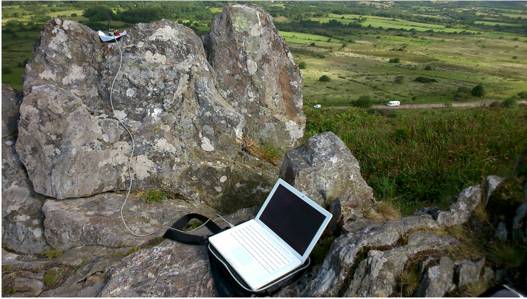
Figure 4.11 – A base station is equipped a RECOCO board (emitter) E.0.1 and a MacBook. This base station was deployed on the top of the Roc’h Trevezel mountain, France. The receiver is another RECOCO board mounted on a car moving around.
