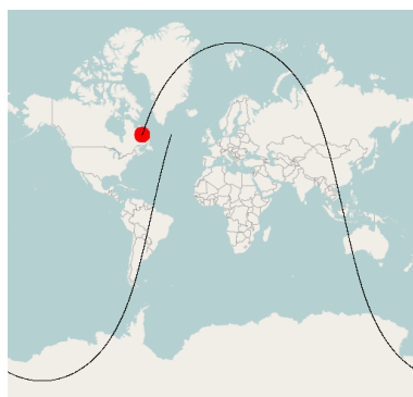
Figure 7.1 – LEO satellite's trajectory westward shifts due to the Earth's rotation [4].
