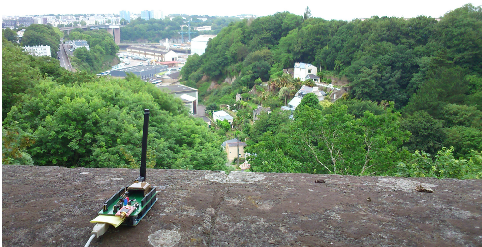
Figure 4.7 – A LoRa emitter was placed on top of a hill at Albert1 er , Brest city, France.
