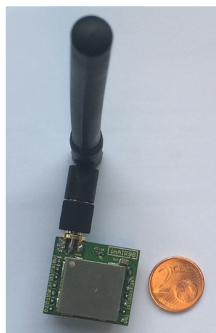
Figure B.1 – LoRa transceiver inAIR9b: Semtech’s chip sx1276, 868-915 MHz [176].
