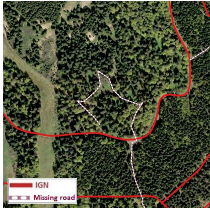
Figure 112 : Road out of authoritative (IGN) data specification
