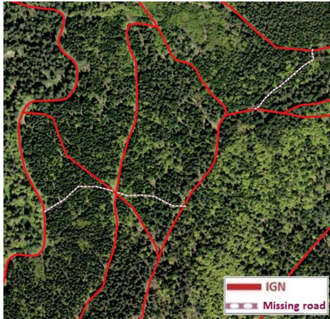
Figure 107 : Real world examples of shortcut roads detected by the approach
