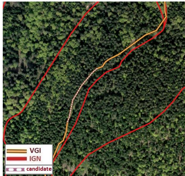
Figure 92 : False positive candidate for missing road
