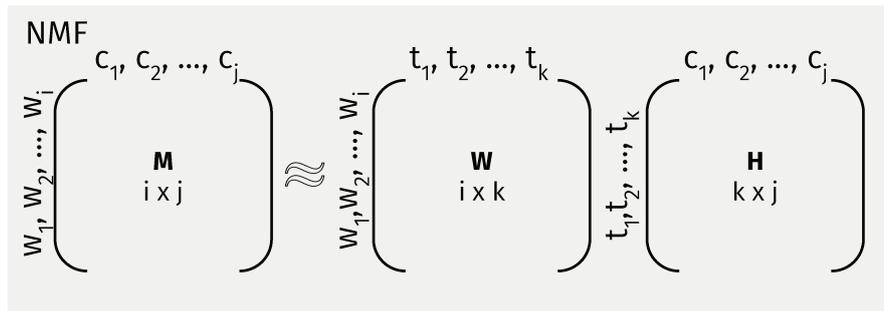
Figure 2.10: Factorization of the matrix  $M$  using NMF. Two matrices are generated:  $W$  and  $H$ .  $W$  contains the words in a  $k$  reduced space.  $H$  contains the contexts in the reduced space.
