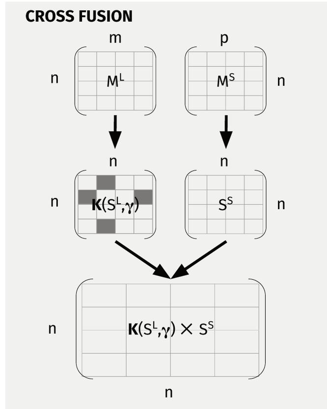
Figure 3.8: Cross fusion for matrices A and B. Similarities are computed, the best similarities are selected for A and finally a product is calculated between the similarities of B and the top similarities of A.
