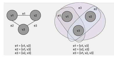
Figure 3.2: A graph (to the left) compared to a hypergraph (to the right). The edges of the hypergraph (hyperedges) may hold more than two nodes at once, relaxing the constraint of graphs' binary relations. A hypergraph can be seen as a set of n-ary sets:  $E = \{\{v1, v3\}, \{v2, v3\}, \{v1, v2, v3\}\}.$
