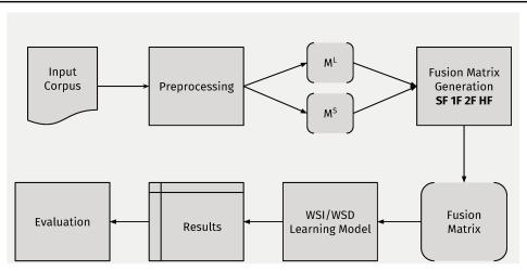
Figure 4.6: Steps followed on our fusion-enriched representation for WSI/WSD experiments. First the corpus is lightly preprocessed, then features are extracted from the text. A fusion matrix is generated, which in turn is used as input to the learning algorithm. Finally, the system yields its results and to be analyzed.
