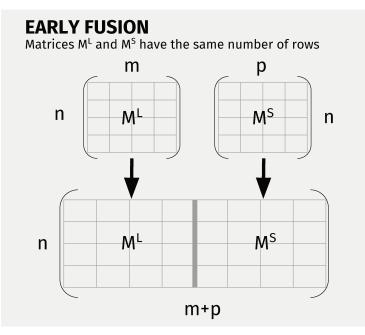
Figure 3.6: Early Fusion of feature matrices A and B. The result is the concatenation of both matrices.
