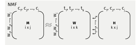
Figure 2.10: Factorization of the matrix M using NMF. Two matrices are generated: *W* and H. *W* contains the words in a k reduced space. H contains the contexts in the reduced space.
