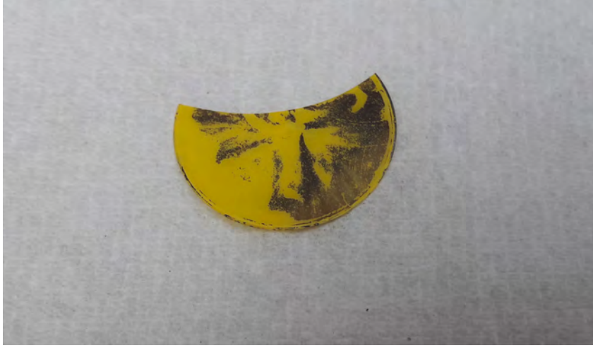
Figure 3.4: A photograph showing decomposed \text{MAPbI}_3 sample with yellow \text{PbI}_2 precipitations.
