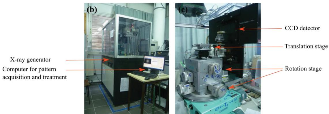
Fig. 4.4 (a) Scheme of the principle of the Laue technique in the back-reflection mode. (b) and (c) Experimental set up with 6-degree of freedom rotation and translation stages.
