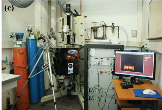
Fig. 3.7 (a) Schematic diagram of optical floating zone apparatus. (b) Stages of nucleation on ceramics rods. (c) Experimental set-up of a mirror furnace at ICMCB.
