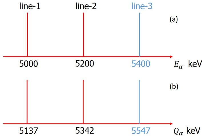
Figure 4.1: Illustration of \alpha -decay spectra where line-1 and line-2 are calibrants and line-3 is unknown at an equal distance from line-2. (a) Case for which the detector detects only the \alpha -particle energy. (b) Case where the detector detects also the recoiling nuclide.
